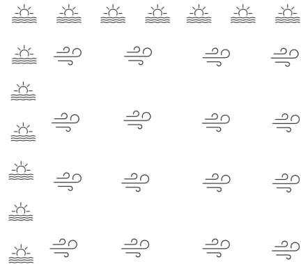
Figure 2.14 - Schematic of the ‘protective’-method. ☀ represents the wind turbines, and 🌊☀ represents either a WEC or an FPV-unit. Inspiration taken from [35].
