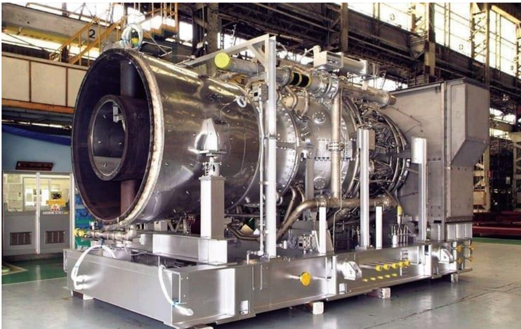
Figure 18; Mitsubishi's H-25 Series gas turbine, intended for use with ammonia. [44]
