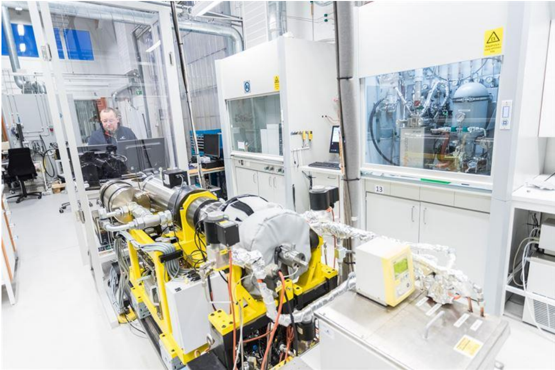
Figure 17; The four-stroke combustion engine Wärtsilä will fuel with ammonia. [43]
