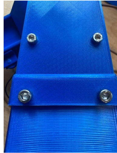
Figure 10 - Bolts connecting the parts
