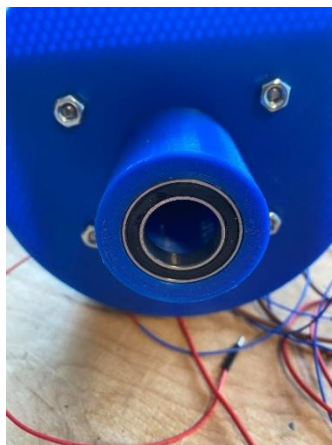
Figure 9 - Bearing in the foot of the crane
