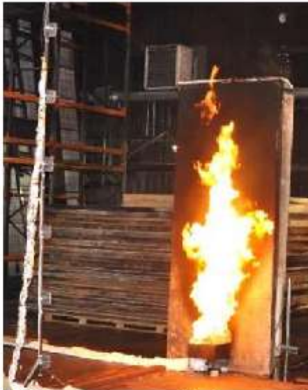
PTHFM mounted on a movable pole to map radiant heat flux around a pool fire
