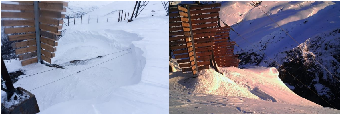
Figure 3-22: Images showing the development of scours around the wind baffles. On the left: The scour was well developed around Baffle nr 1 during fieldwork 06.03. On the right: Image from Cam 4 showing the scour around baffle 1 on the ridge side. Note the increased snow height on the lee side of baffles 3 and 4 in the background.
