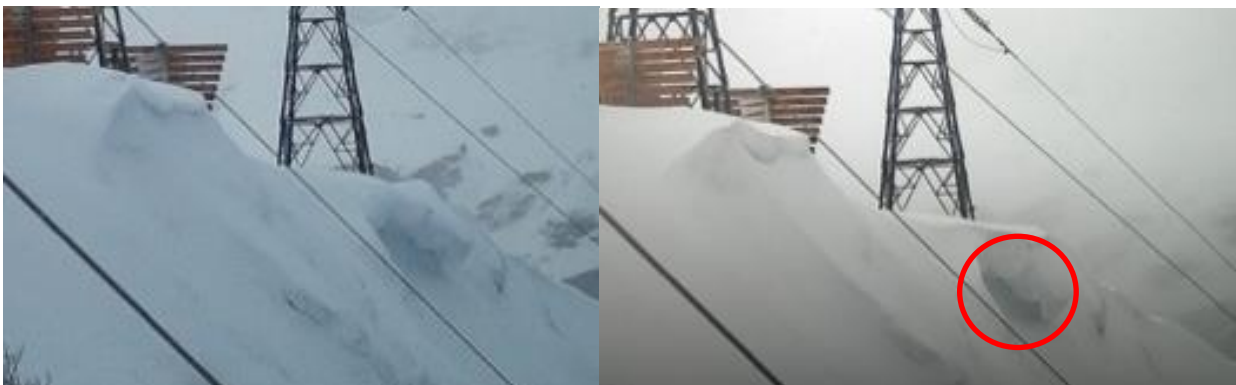
Figure 3-9: By 15.03 the cornice face had almost deformed enough to create a roll cavity (red circle). Images from Cam2 09.03 (left) and 15.03 (right).
