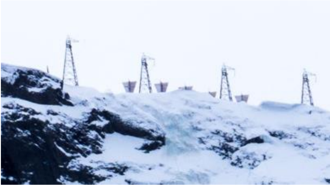
Figure 3-21: The ridgeline at Kvannberget seen from below. No continuous cornice had developed by 06.03.20. The cornice structure seen between the two masts on the right was used as the reference cornice. Image taken during field work 06.03.20
