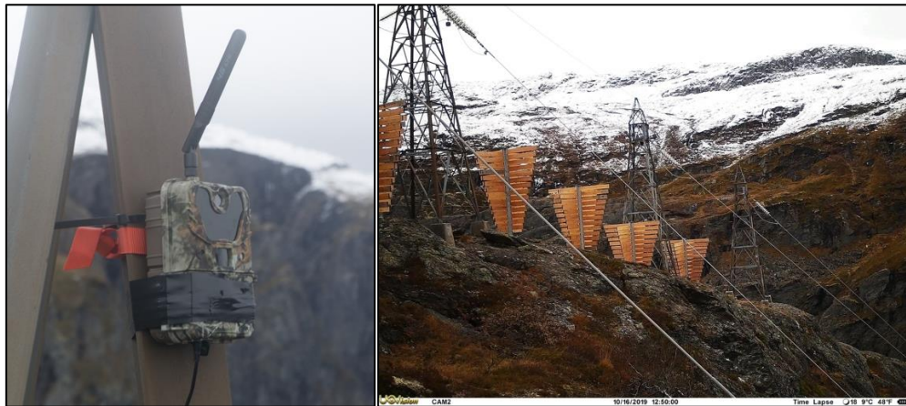
Figure 2-8: Left: The Uovision UM785-4G with external antennae to increase reception. Right: Example of an image downloaded through the cloud service. This feature was used several times to check if the cameras were operating normally.
