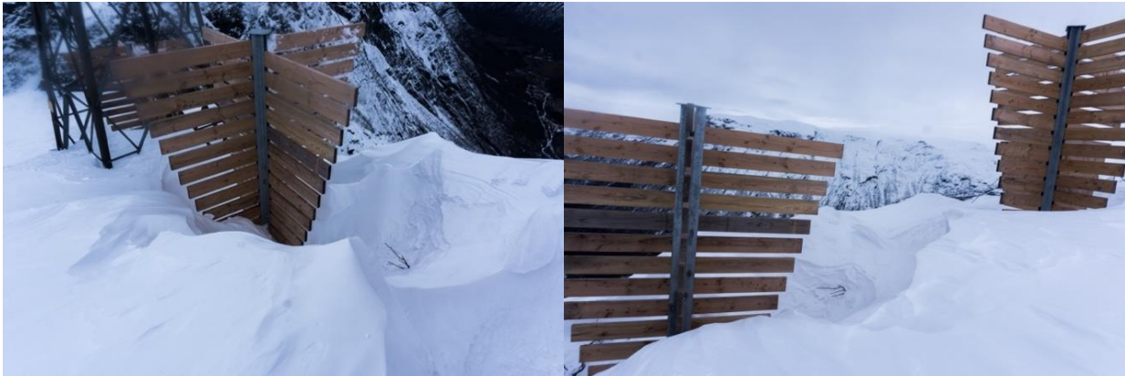
Figure 3-23: Snow had deposited on the lee side of baffles 3 and 4. On the left: The scour around baffle 4 was notably smaller than the other scours. Snow had deposited in contact with the bottom of the baffle. An elevated snow surface can be seen between the scour around baffle 4 and 3 (to the right of the frame). On the right: Snow had deposited on the lee side of baffle 3 (right) and 4 (left). Snow height on the windward side of baffle 4 was notably higher than for baffle 3.
