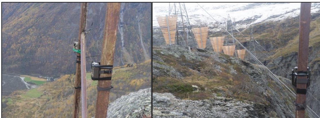
Figure 2-7: Two cameras were placed on a ridge to the North of the wind baffles and provide a view over the area previously subjected to cornice growth, as well as the control area. The cameras were pointing southwards.
