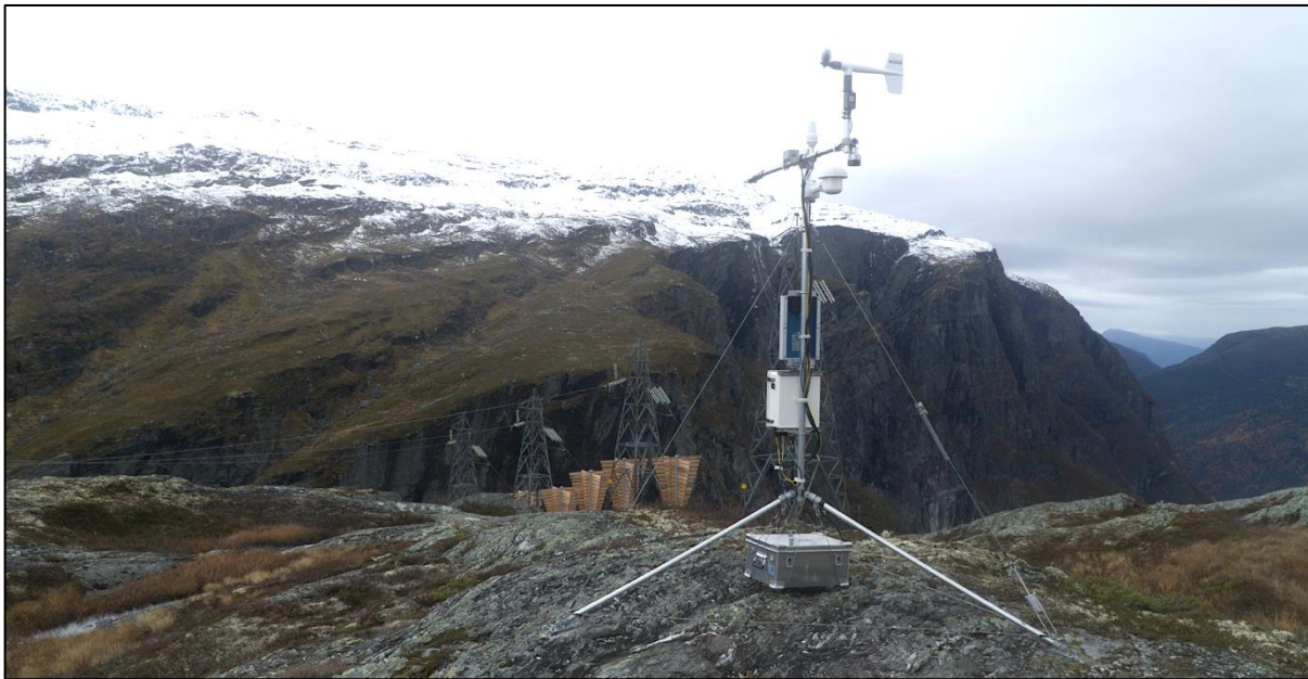
Figure 2-6: The automatic weather station was placed to the Northeast of the wind baffles on an elevated surface. Wind measurements were made at a 3.1m height by the anemometer seen on top of the boom. The boom is mounted in a North-South orientation.
