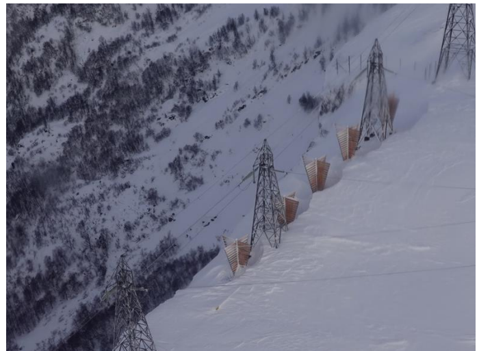
Figure 4-2: Aerial image of the field site taken 27.02.20. A distinct decline of the snowpack can be seen windward of the baffles.
