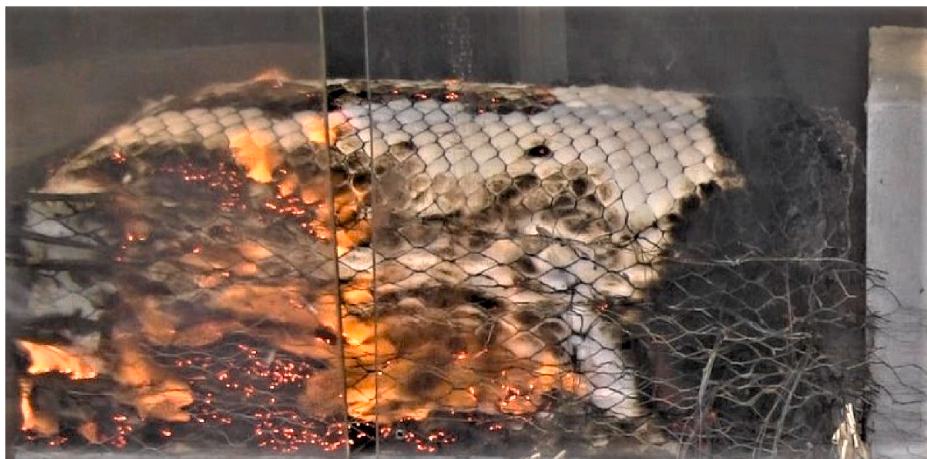
Fig. 7. Flames have spread from the inside to the outside of the sample. Sample size is 0.6 \text{ m} \cdot 0.4 \text{ m} \cdot 0.15 \text{ m} , with density 80 \text{ kg/m}^3 . This type of flame spread initiated smoldering on a large portion of the surface of the sample, resulting in more erratic temperature increase in the sample.
