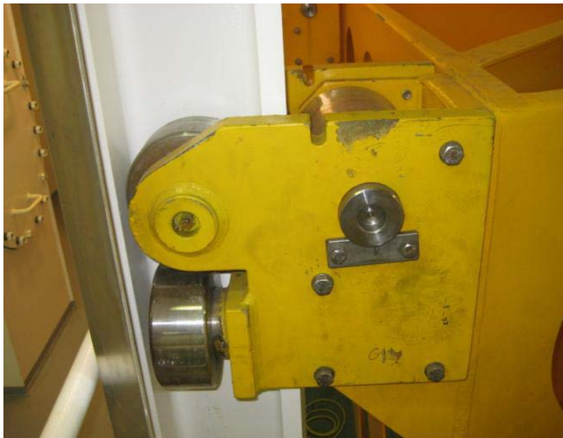
Figure 9: Vertical guiding of cursor system design.
