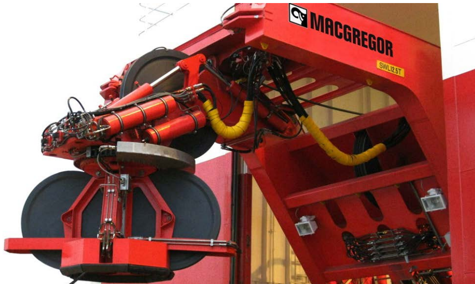
Figure 1: Example of LARS over the side, Macgregor [5]
