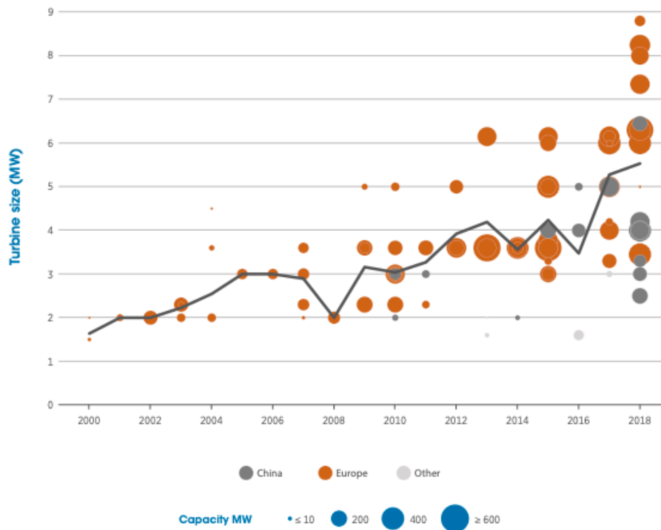
Figure 6 - Turbine size for commissioned offshore wind projects and global weighted average (2000-2018) [5]
