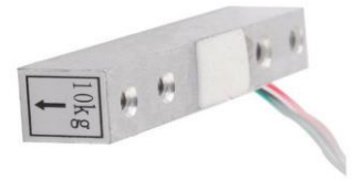
Figure 3-2, The load cells used in this experiment is made to measure forces as high as 10kg
