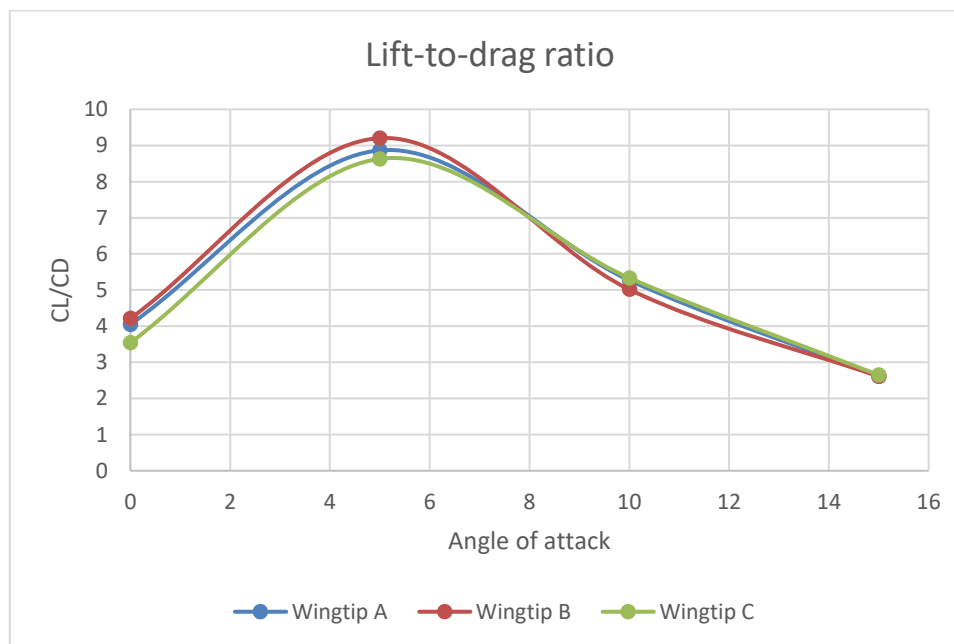
Figure 5-9, Lift-to-drag ratio for different wingtips at velocity at 1,5m/s
