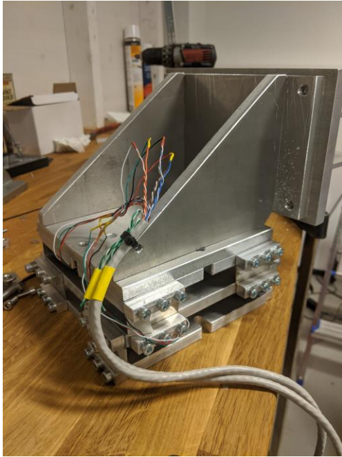
Figure 3-5, The load cell configuration can measure forces in horizontal and vertical direction
