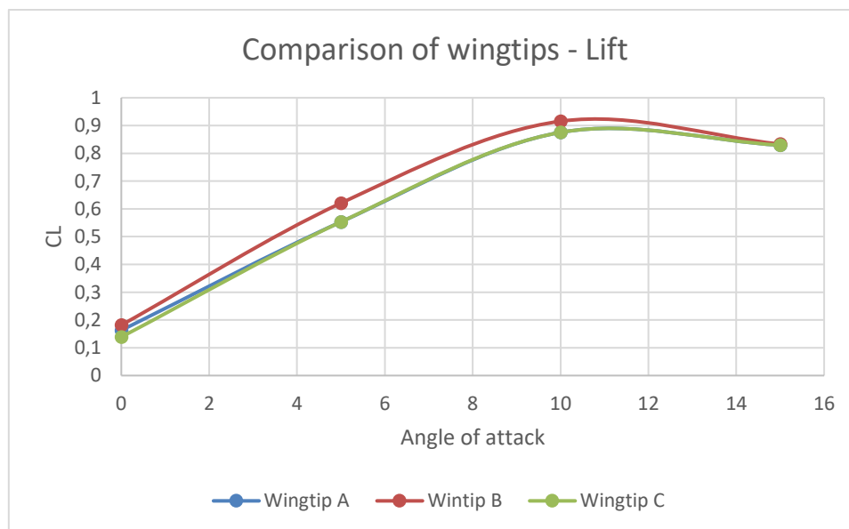
Figure 5-7, Different types of wingtips compared for lift at different angles. Velocity at 1,5m/s
