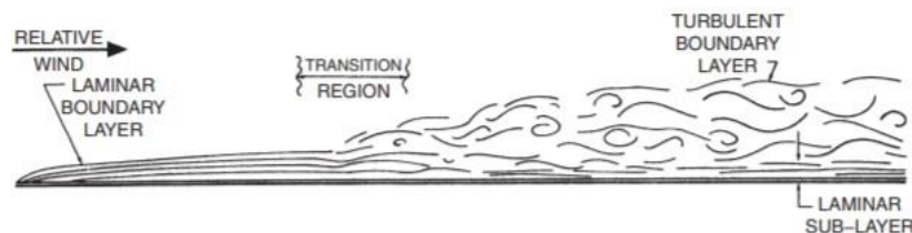
Figure 2-7. Boundary layer composition
