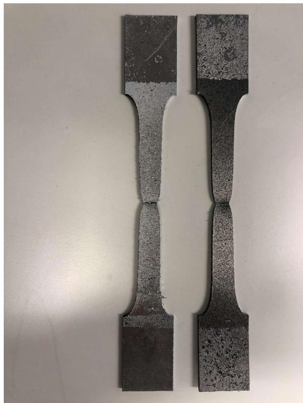
As mentioned in the previous chapter, the white paint broke. After this, the possibility of spraying the pattern directly onto the metal surface was tried out, as it is shown in Figure 25, giving good enough quality in the surface component generated by the software.
