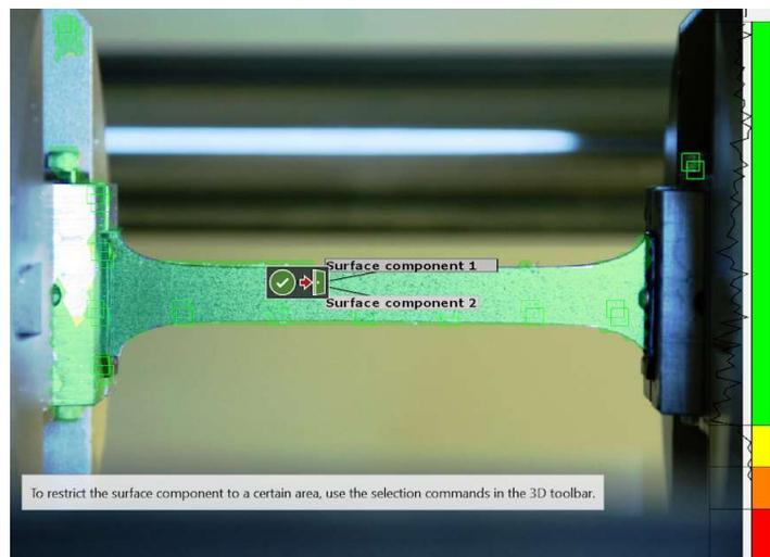
Even though the non-acceptable areas increase slightly (yellow and orange), the great majority of our surface component is still good enough to carry out our test with GOM Correlate. The white areas, where the software is not able to calculate the strain, are increasing slightly.
