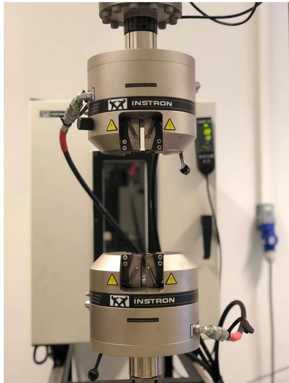
*Figure 2: Tensile machine*
