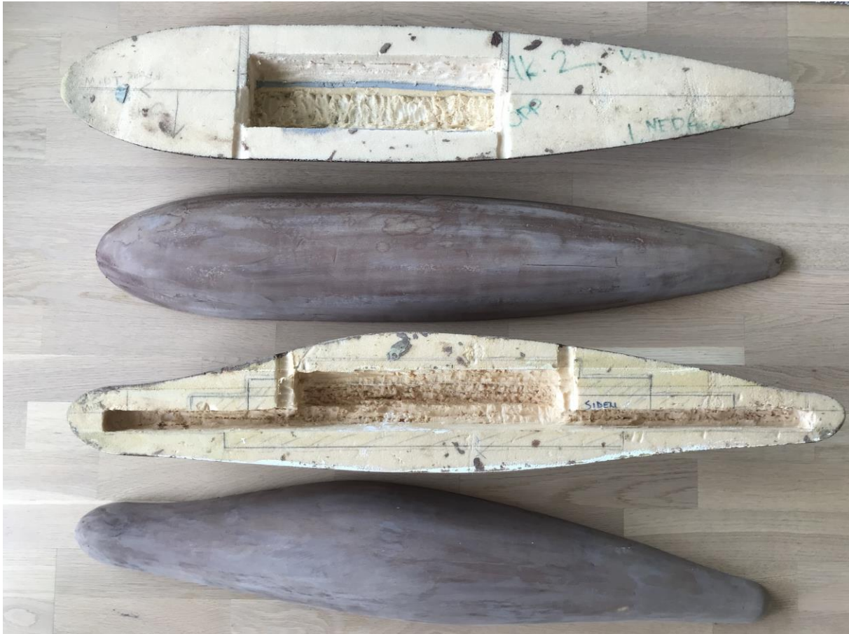
Figure 29: Drone hull halves with space for ballast rods, after epoxy and sanding.
