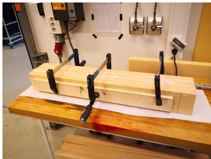
Figure 26: Divinycell plates after gluing, preparing for further treatment.
