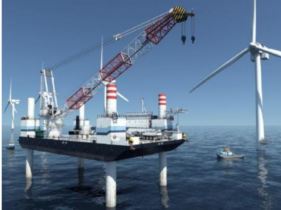
Figure 48 Rendered Image of a Jackup Barge in Operation (offshorewindbiz, as cited in Kopits and Losz, 2013)
