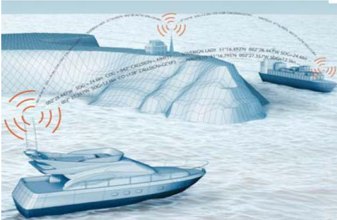
Figure 36 AIS Systems Sharing Information (Kopits & Losz, 2013).
