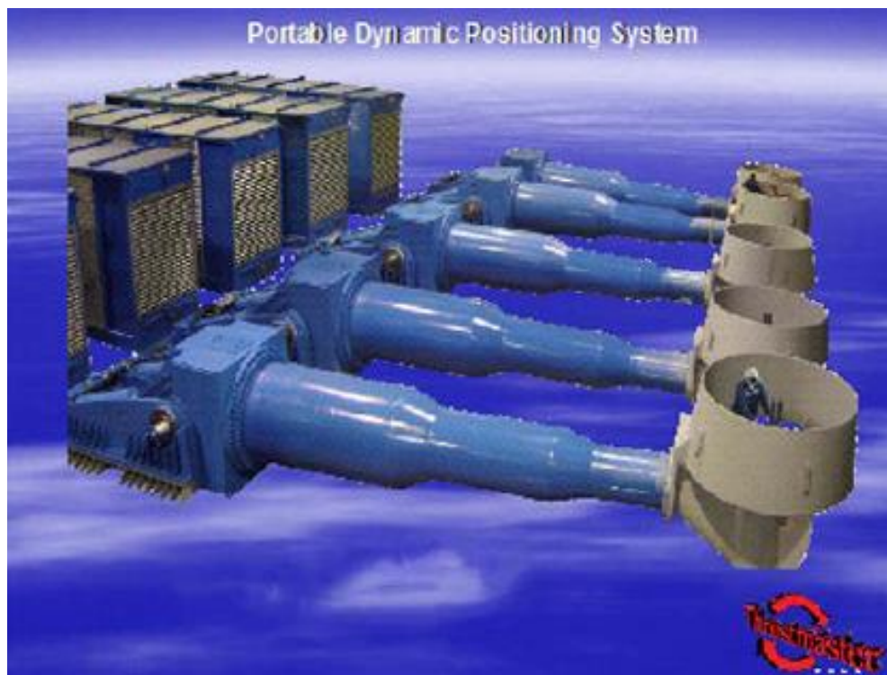
Figure 32 Portable Dynamic Positioning System (Kopits and Losz, 2013).
