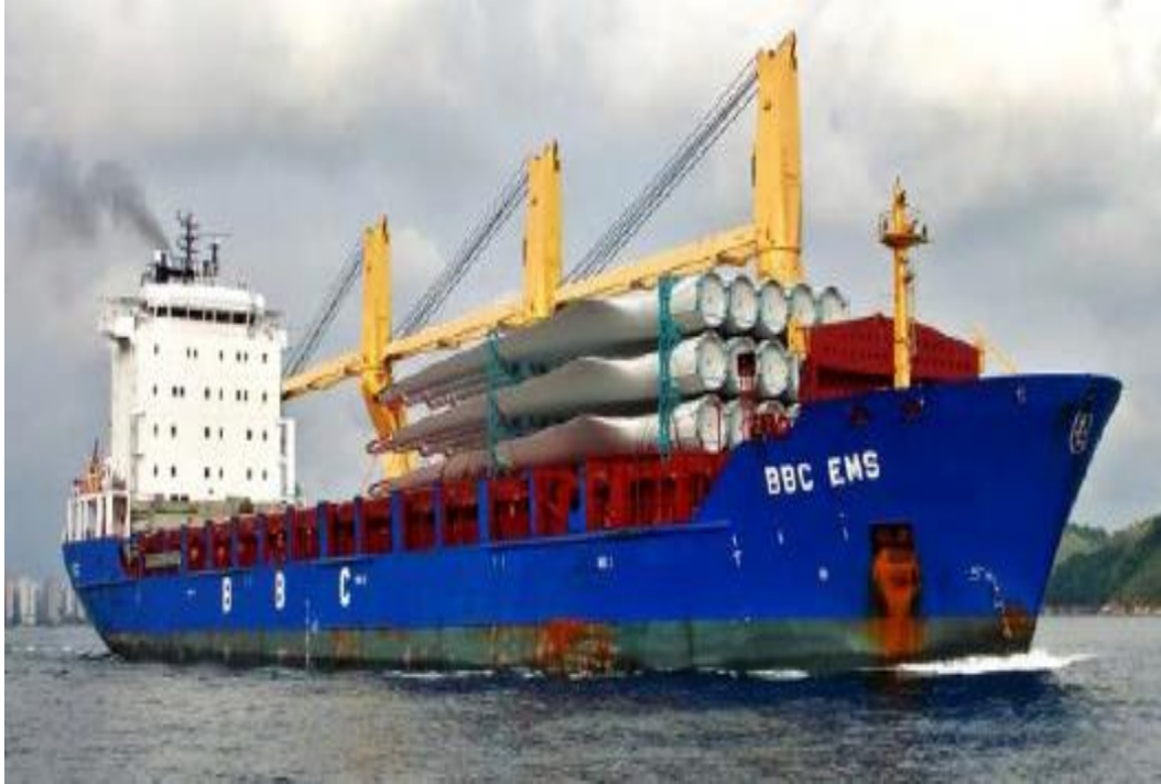
Figure 46 Heavy Lift Vessel with a Load of Turbine Blades (Kopits & Losz, 2013)
