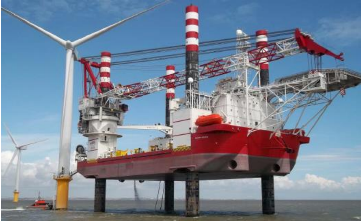
Figure 40 Columnar Jackup Legs (Kopits and Losz, 2013).
