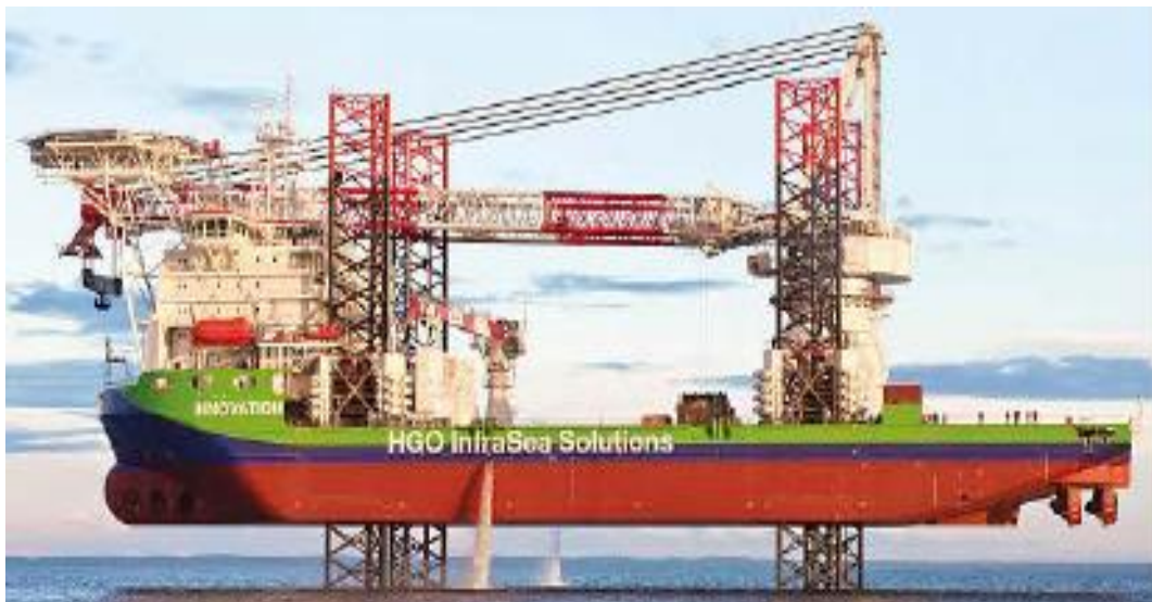
Figure 39 Open Truss Jackup Legs (Kopits & Losz, 2013).
