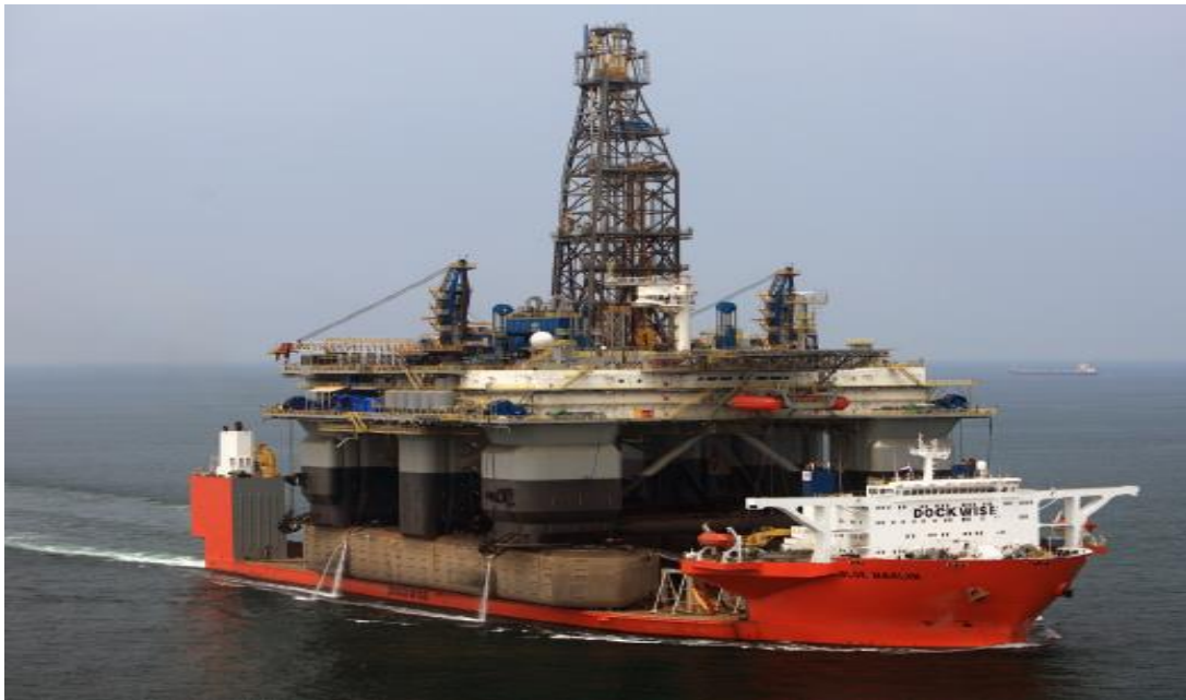
Figure 45 Semi-Submersible Heavy Lift Vessel Transporting an Offshore Platform (Kopits & Losz, 2013)
