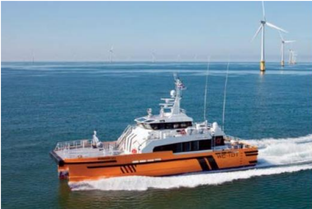
Figure 54 Motion Stabilized Personnel Transfer Vessel (Kopits & Losz, 2013)
