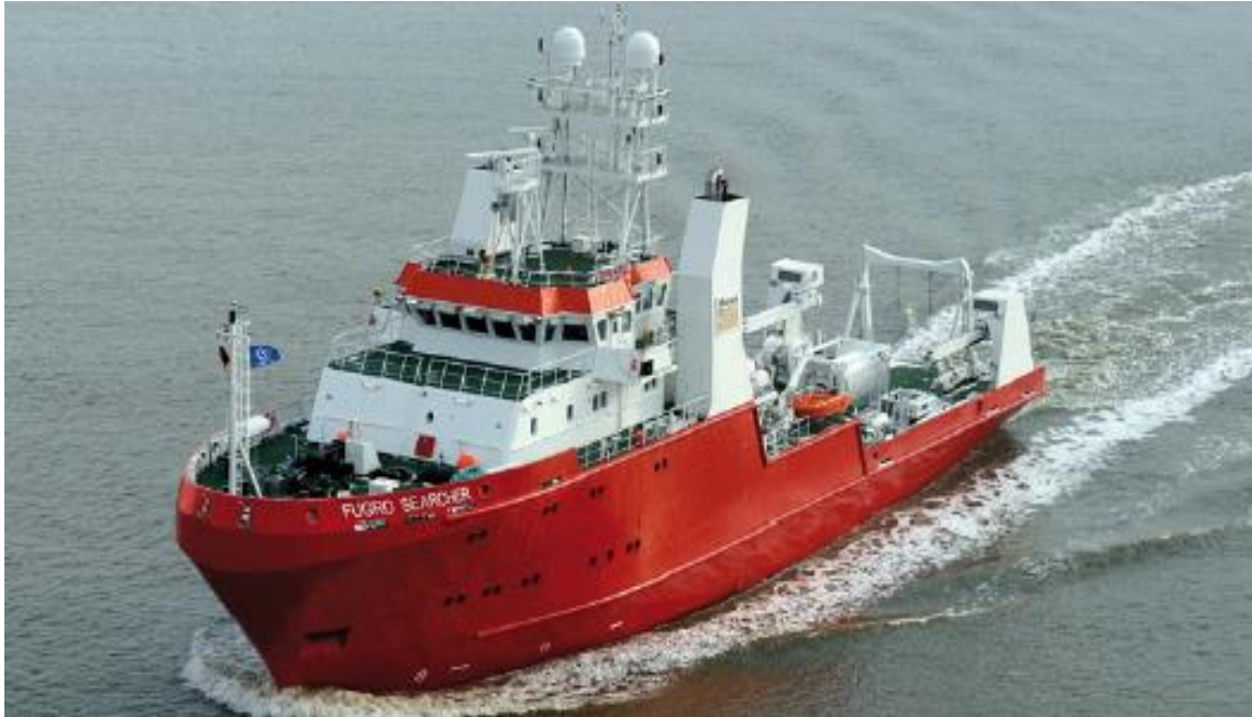
Figure 51 Fugro Searcher Offshore Survey Vessel Designed for Geophysical Research (Kopits & Losz, 2013)
