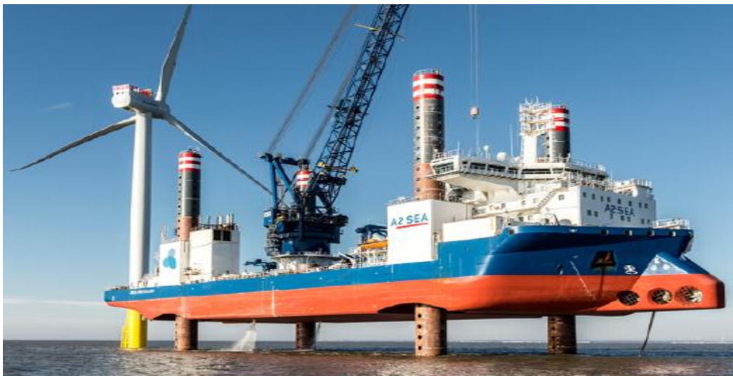
Figure 44 TIV at Sheringham Shoal (World Maritime News as cited in Kopits and Losz, 2013)
