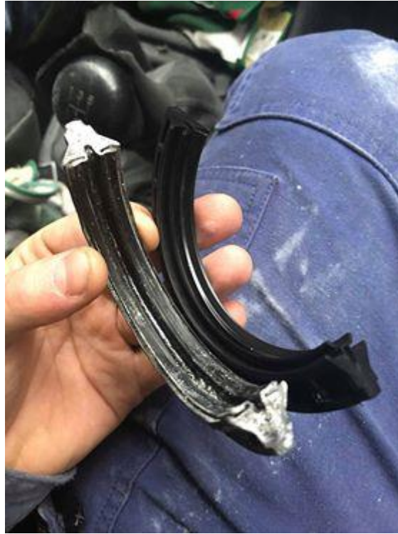
Figure 5. 12: A worn out seal next to a new one
