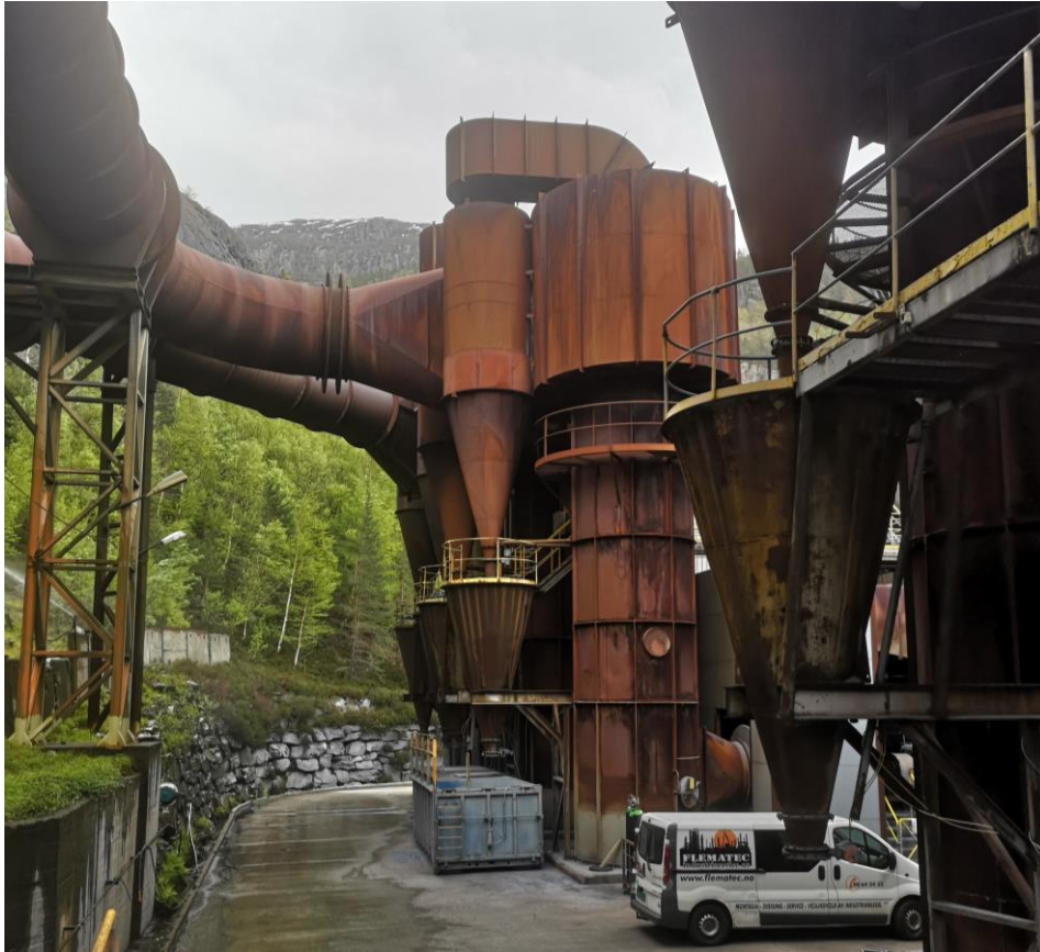
Figure 4. 3: Sub-system - coarse separator
