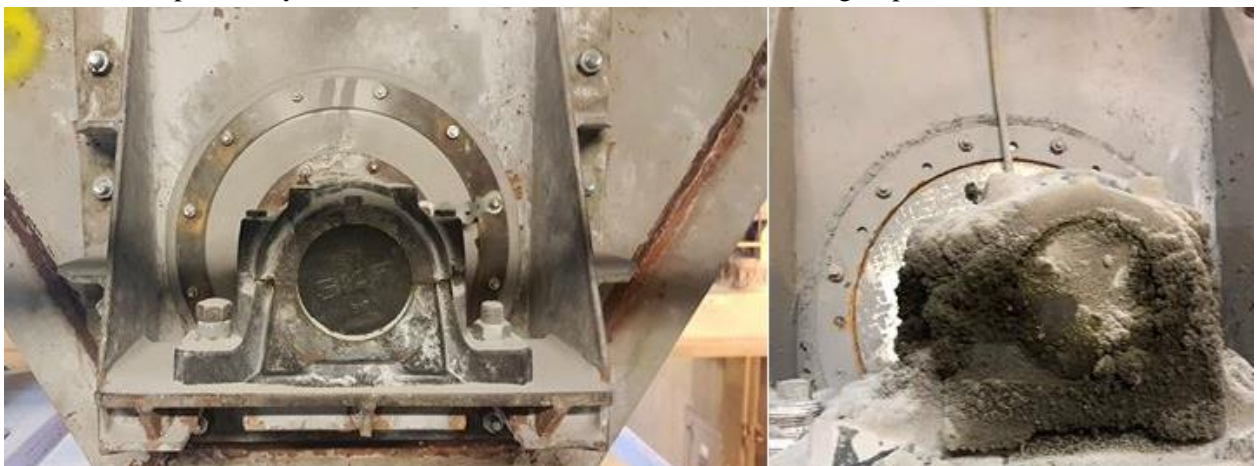
Figure 5. 9: Clean vs dirty bearing house
