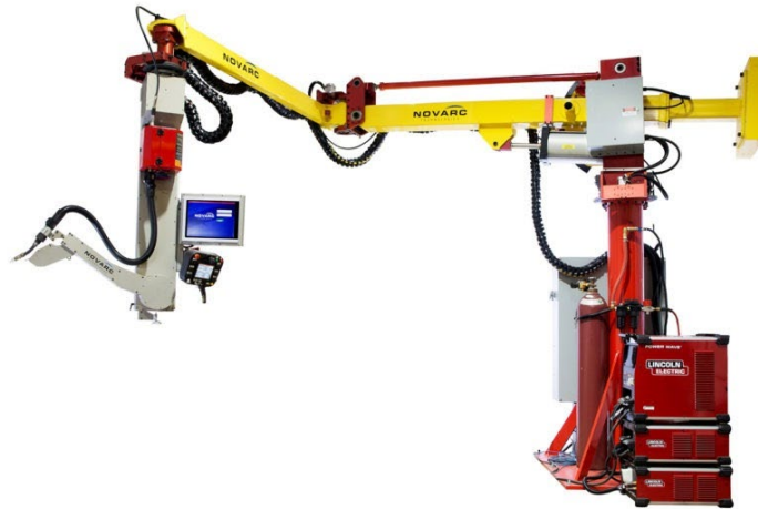
Figure 8. Novarc collaborative welding robot [18]
