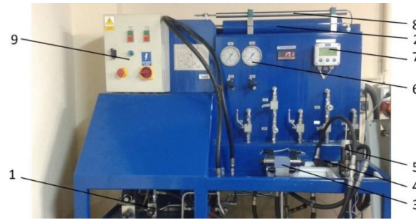
Fig. 5. Test bench front view; 1 – safety valve, 2 – hydraulic cylinder, 3 – control valve, 4 – check valve, 5 – relief valve, 6 – p_1 pressure gauge, 7 – flow meter display, 8 – displacement transducer, 9 – control panel
