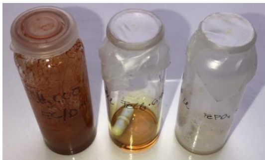
Figure 36. Electrolytes based on 1 M Fe(CH 3 COO) 3 , FeCl 3 and FePO 4 in DMC+EC, respectively from left to right.
