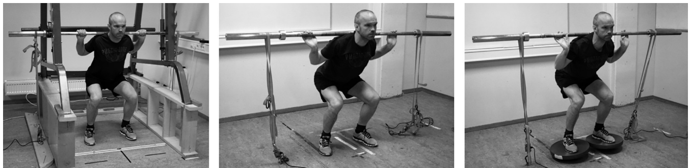
Fig 2. Testing procedures for the RFD, EMG and MVIC with low stability requirement, medium stability requirement and high stability requirement.
