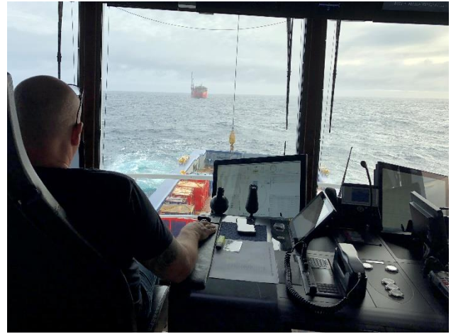
Figure 3. Officer in stern steering position. A thruster-lever and the DP joystick can be seen in front of the screen ahead. The touch-panel with integrated functions is facing toward the officer on his right-hand side.
