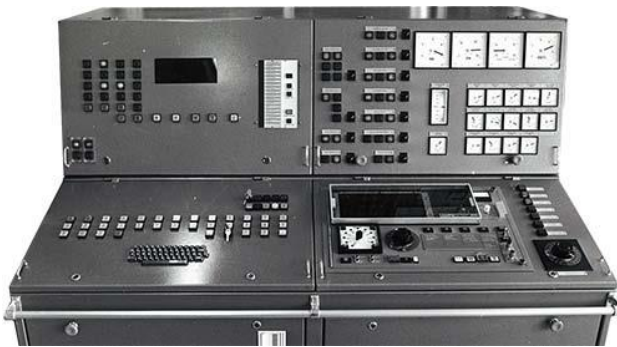
Figure 3: The Norcontrol analogue diesel engine simulator delivered to Trondheim Maritime College in 1978 (Kongsberg Maritime, 2019).
