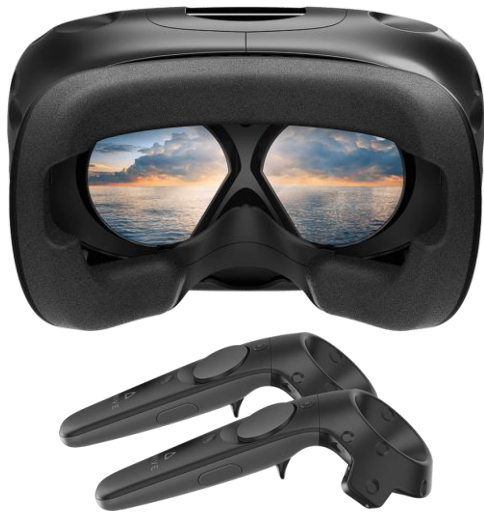
Figure 7: HTC VIVE head mounted device, and hand controllers of the immersive VR simulator
