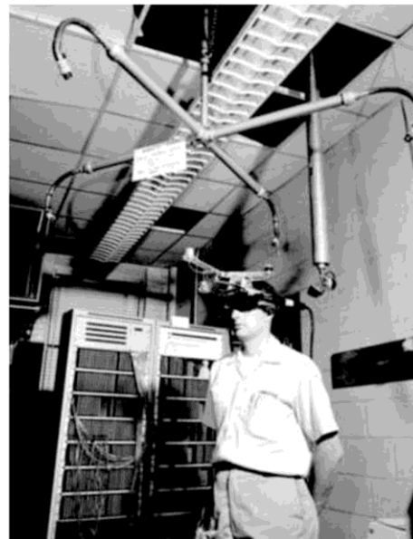
Figure 3 Sword of Damocles by Ivan Sutherland (First computer connected VR system)
