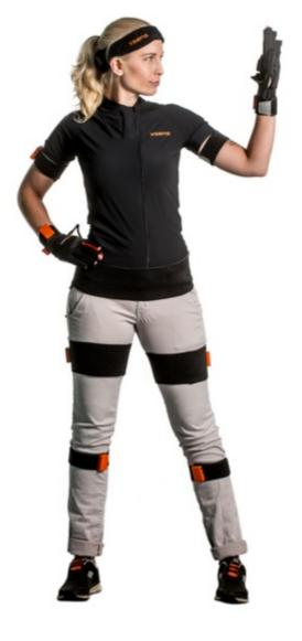
In this project, it is investigated the use of Inertial Measurement Units (IMUs) to solve these corresponding issues. Instead of using often preferred camera based systems it is proposed a wearable motion capturing system using IMUs.
