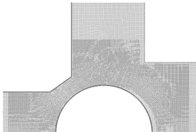
Fig. 6. Overset mesh model for safety valve presented in Fig. 1.
