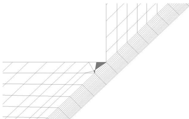
Fig. 2. Problem with quality of cells (cells distortion) during grid deformation (Domagala, 2008)
