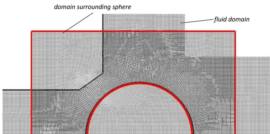
Fig. 5. Overset mesh model for safety valve presented in Fig. 1.
