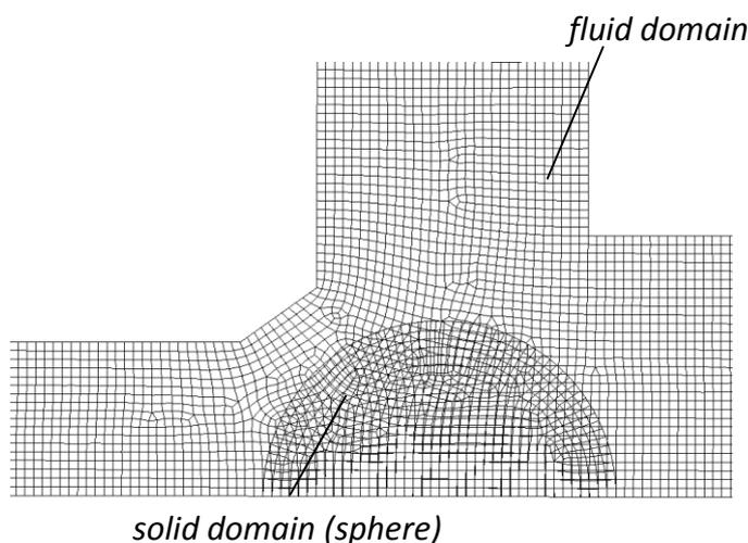
Fig. 3. Lattice nodes for direct operating relief valve (Domagala, 2016)
