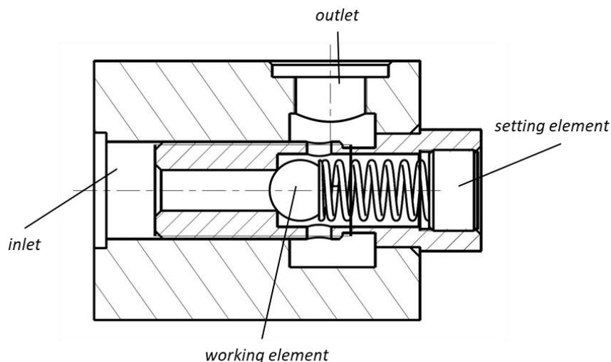
Fig. 1. Simplified drawing of direct acting relief valve
