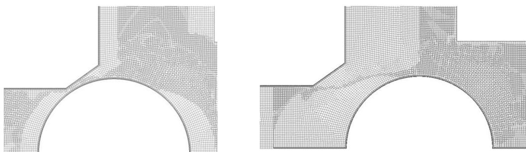
Fig. 7. Grid interface between two fluid domains.
