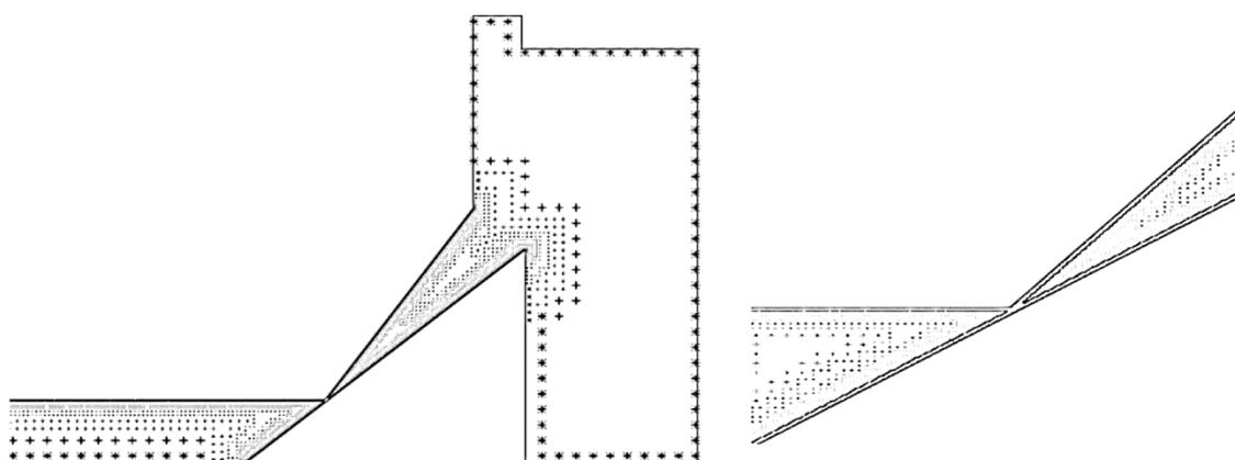
Fig. 4. Lattice nodes for direct operating relief valve (Domagala, 2016)
