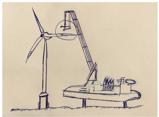
*Figure 12: Sketch - Cutting of turbine blades. Circled area in the next figure.*
