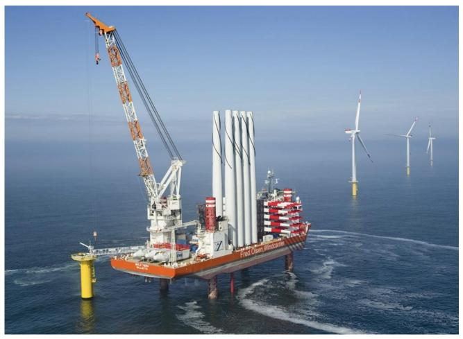
Figure 8: Fred. Olsen Windcarrier installing monopile, fixed-bottom OWT [13].
