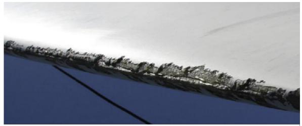
*Figure 10: Leading edge erosion on turbine blade, occurring following small scratches in the surface [31].*
