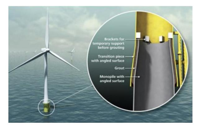
Figure 5: Transition piece, tower, nacelle and blades [25]. Downloaded from 4C Offshore 18th of February.
