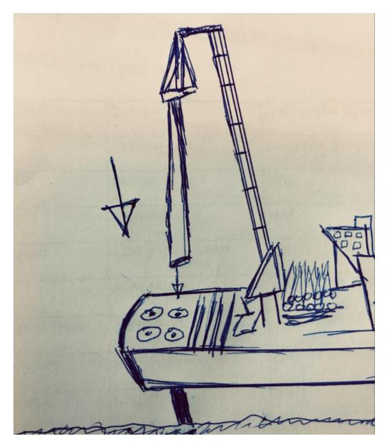
Figure 14: Sketch - Close-up of putting the tower onto the plug at the aft deck of the lifting vessel.
