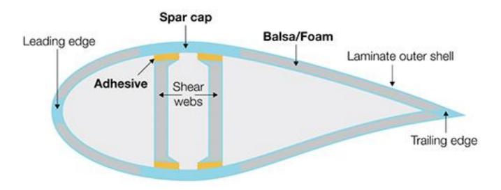
Figure 15: Cross-section of turbine blade [32].
