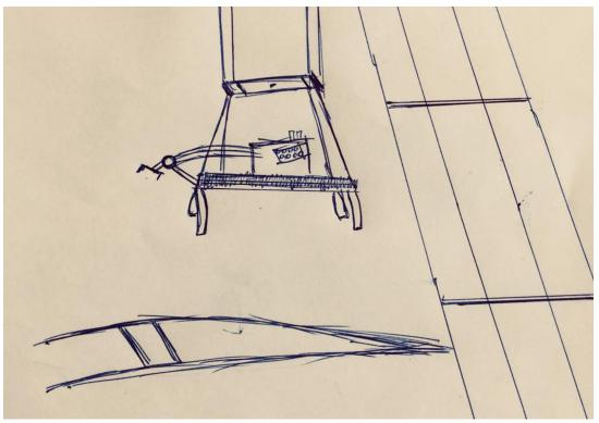
Figure 11: Sketch - Close-up of lifting jig and imaginary motor and cutter. Clutching the blade and at the same time cutting it off. Cutting-mechanism not defined, as this depends on future trends and economic viability.
