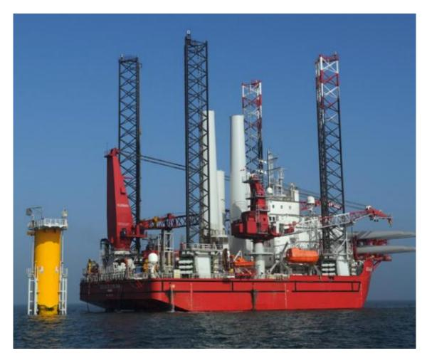
Figure 9: Jack-up vessel "Seajacks Leviathan" loaded with tower and blades, next to an monopile fitted with the yellow transition piece [3].
