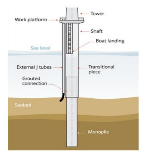
*Figure 4: Monopile foundation [25]. Downloaded from 4C Offshore 16<sup>th</sup> of February.*
