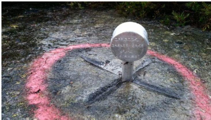
Figure 1. The typical boundary mark in rural areas prior to 1980, cross in bedrock, renewed with the new aluminium boundary marker introduced in 1980. Photo: L. B. Mjøs
