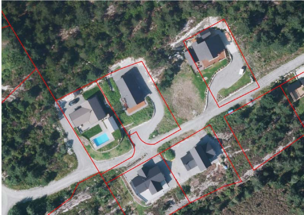
Figure 2. “Legally binding boundaries” based on the zoning plan. The location of the road in the terrain deviates from the plan (Mjøs and Leiknes 2017)
