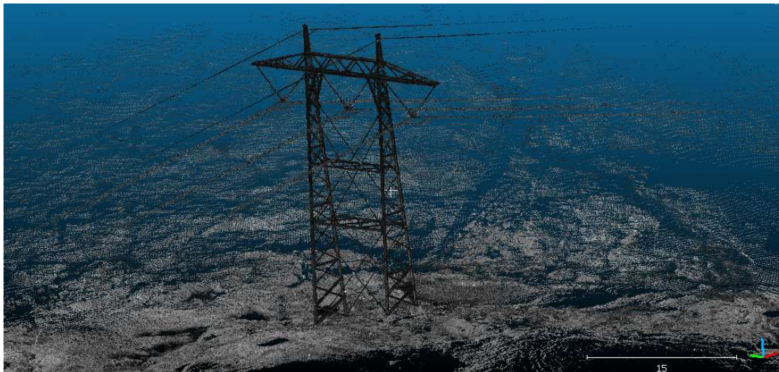
Figure 36: Zoomed in picture of the electricity pylon from the laser scanner (Cloudcompare)
