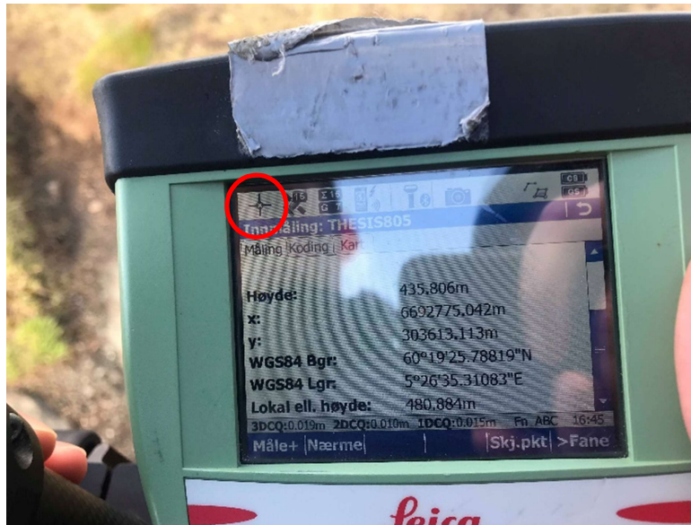
Figure 22: Symbol for fix solution (obtained using CPOS) on the Leica Viva CS10
