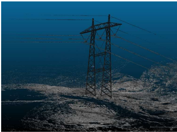
Figure 31: Point cloud own measurement with a terrestrial laser scan data (Cloudcompare)
