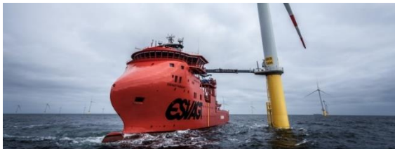
FIGURE 2. Ship servicing a windmill, different methods for stabilization are currently used in todays marked. [4]
