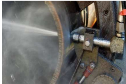
Figure 30 - Abrasive water jet cutting [56]
