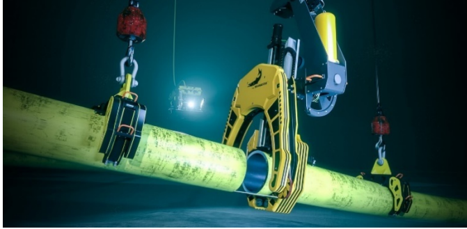
Figure 31 – Diamond Wire Cutting Illustration [19]
