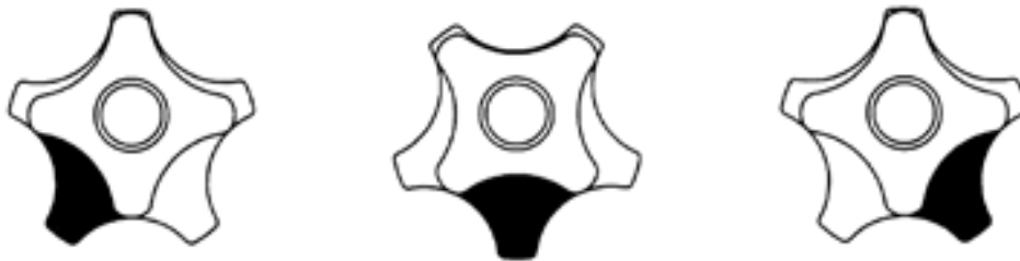
Figur 22 Prinsipp gerotorpumpe, Parker
