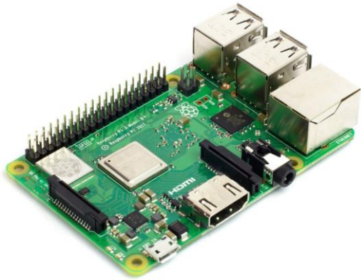
Figur 15: Raspberry Pi 3b+
