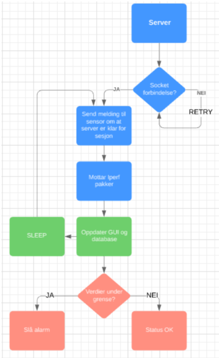
Figur 4.8: Flowchart for server
