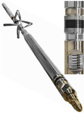
Vernier looks sideways of the tube, gives another view than Focus and Panorama. Main applications of them is: ID evaluation/Caliper, Pipe thickness evaluation, Corrosion logging and Metal loss evaluation.
