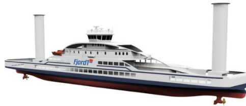
Figure 1: Fjord 1 ferry with Flettner rotors (Fjord 1 ASA)
