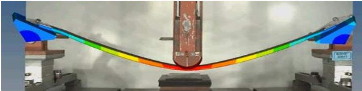
Figure 5. Validation of the simulation model compared to the experiment (reference crash-beam)
