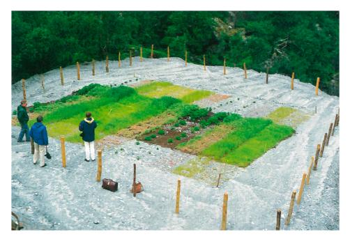
**Figure 3.** A multitude of experiments involving addition of soil, fertilizers and seeds were carried out from the 1960s and onwards to identify optimal restoration methods for spoil heaps. Ulla-Førre, Rogaland, SW Norway. 1985. Photo credit: Knut Ove Hillestad/Norwegian Water Resources and Energy Directorate.
