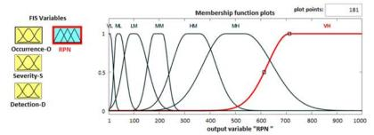
Fig. 5. Fuzzy sets defined for RPN factor using Gauss-type membership functions.
