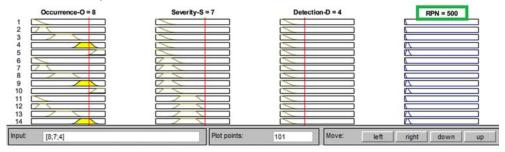
Fig. 6. Fuzzy FMEA system output for S = 7, O = 8, D = 4.
