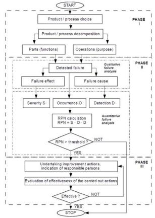
Fig. 1. Process of a conventional FMEA analysis.
