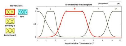
Fig. 3. Fuzzy sets defined for Occurrence factor using Gauss-type membership functions.
