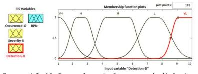
Fig. 4. Fuzzy sets defined for Detection factor using Gauss-type membership functions.
