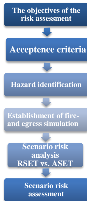
Figure 12 - Schematic process of the risk assessment used in this study [Figure by Emmanuel Eriksson]
