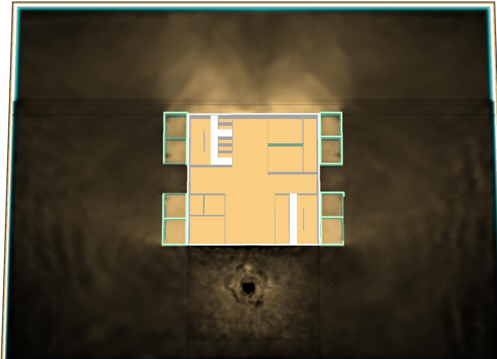
Figure 24 - Smoke development and visibility level at 272 s in design fire 3 simulation in the Swedish high-rise
