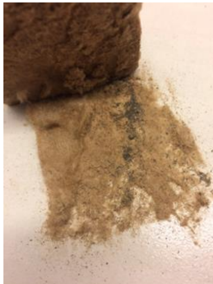
Figure P. 4 Insulation specimen after heating up to 750 °C.
