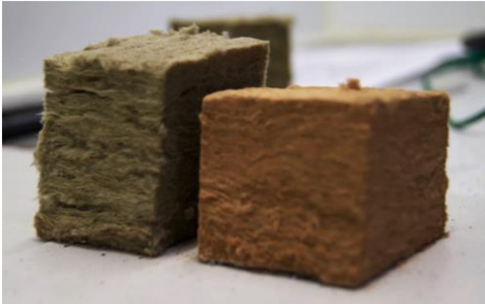
Figure P. 1 Insulation specimen before (to the left) and after (to the right) the oven testing. The picture to the right is the insulation specimen after the test with a set temperature of 900 °C.
