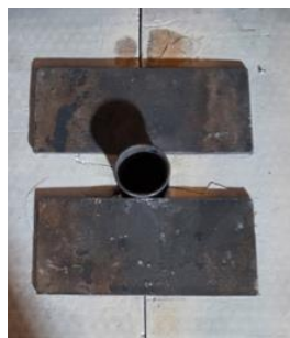
Figure B. 4 Location of the steel plates around the burner.
