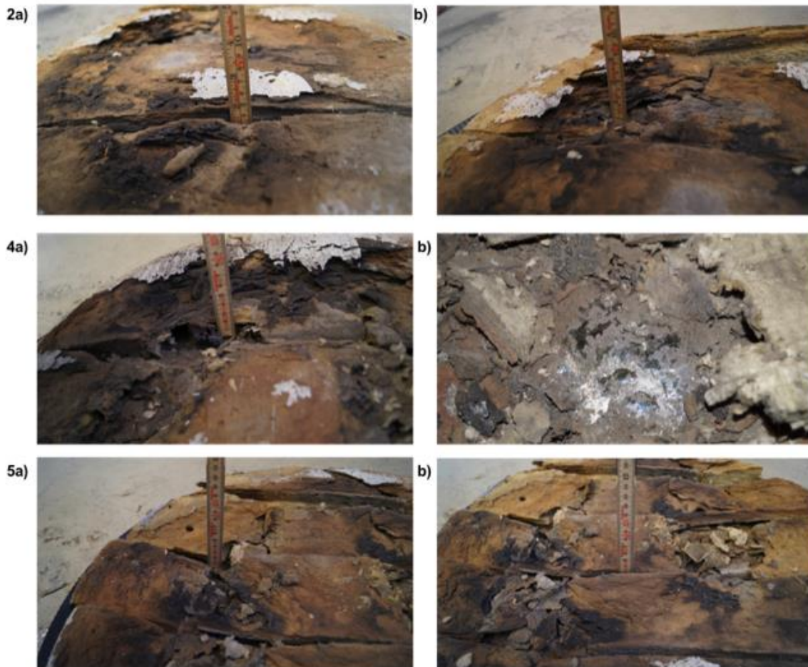
Figure 5.5 Close-up photos of the insulation after testing.
