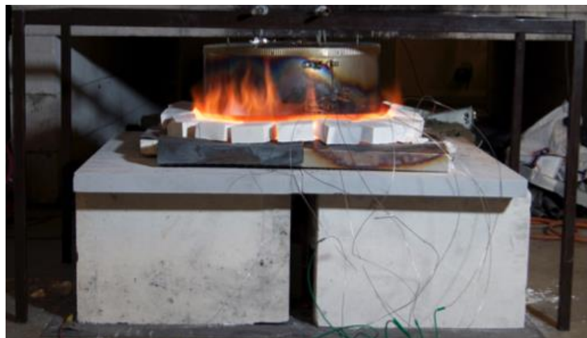
Figure 3.8 Horizontally suspended test unit during fire exposure. The picture is taken during test 17.
