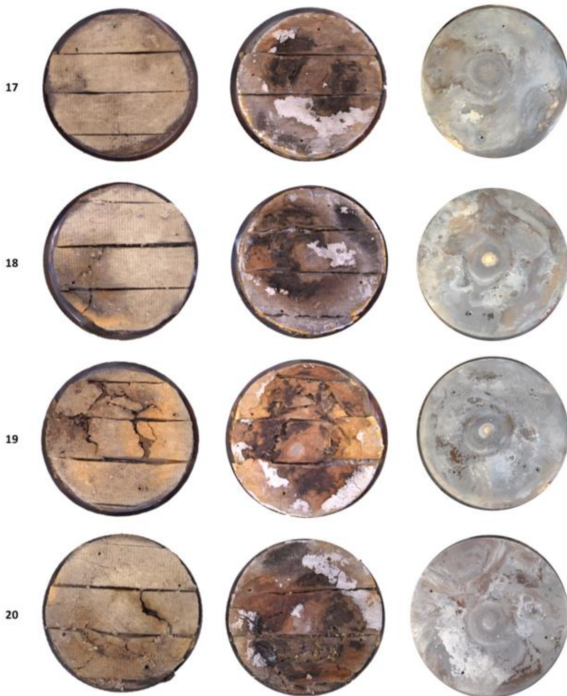
Figure I. 13 Insulation after testing for test 17, 18, 19 and 20. The column to the left shows the unexposed side of the insulation after testing, the middle column shows the exposed side of the insulation after testing, and the column to the right shows the exposed cladding. Each row represents one test.
