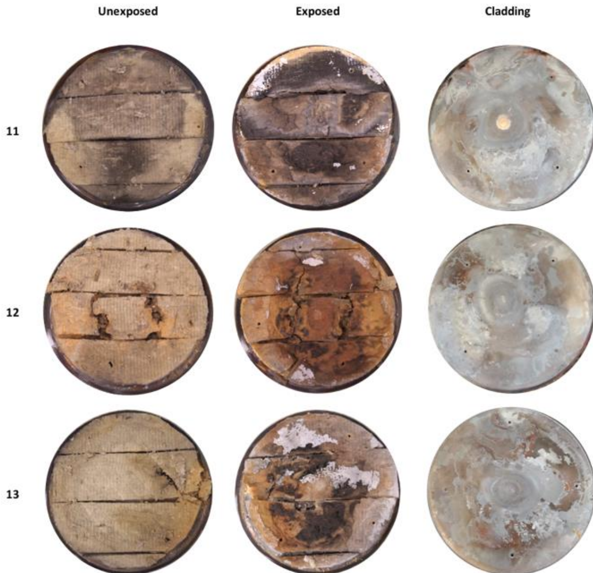
Figure I. 9 Insulation after testing for test 11, 12, and 13. The column to the left shows the unexposed side of the insulation after testing, the middle column shows the exposed side of the insulation after testing, and the column to the right shows the exposed cladding. Each row represents one test.
