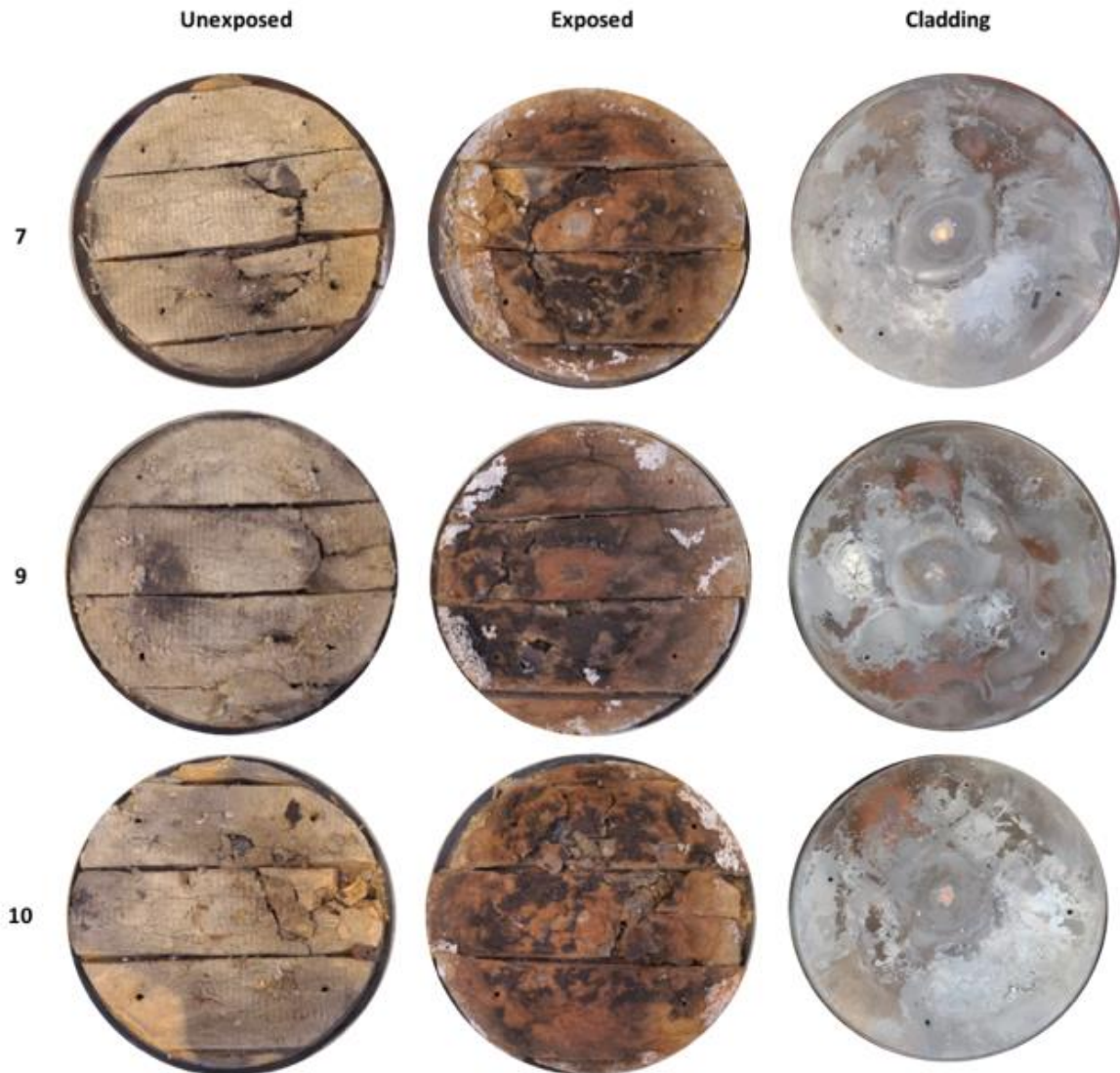
Figure 5.9 Insulation after the testing for test 7, 9 and 10, with a 12 mm steel plate thickness. Each row represents one test, The unexposed side of the insulation, the exposed side of the insulation and the exposed side of the bottom cladding.
