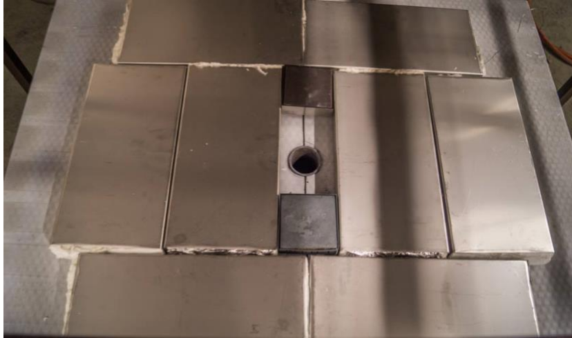
Figure B. 5 Location of cladding boxes, burner and plate thermometers, seen from above.
