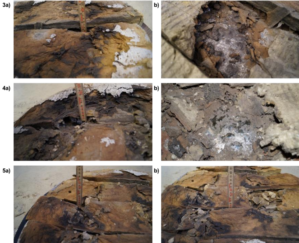
Figure I. 4 3a and b) Insulation after test 3. 4a and b) insulation after test 4. 5a and b) Insulation after test 5.
