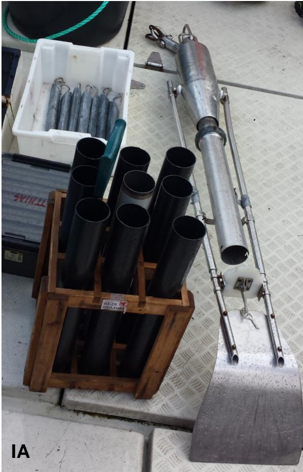
Figure 1a: Niemistö (1974) Gravity Corer (Meskanen, 2017)
