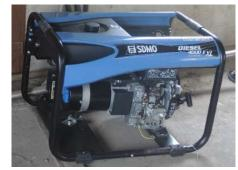
Figure 4.15 - 4-kVA SDMO Generator
