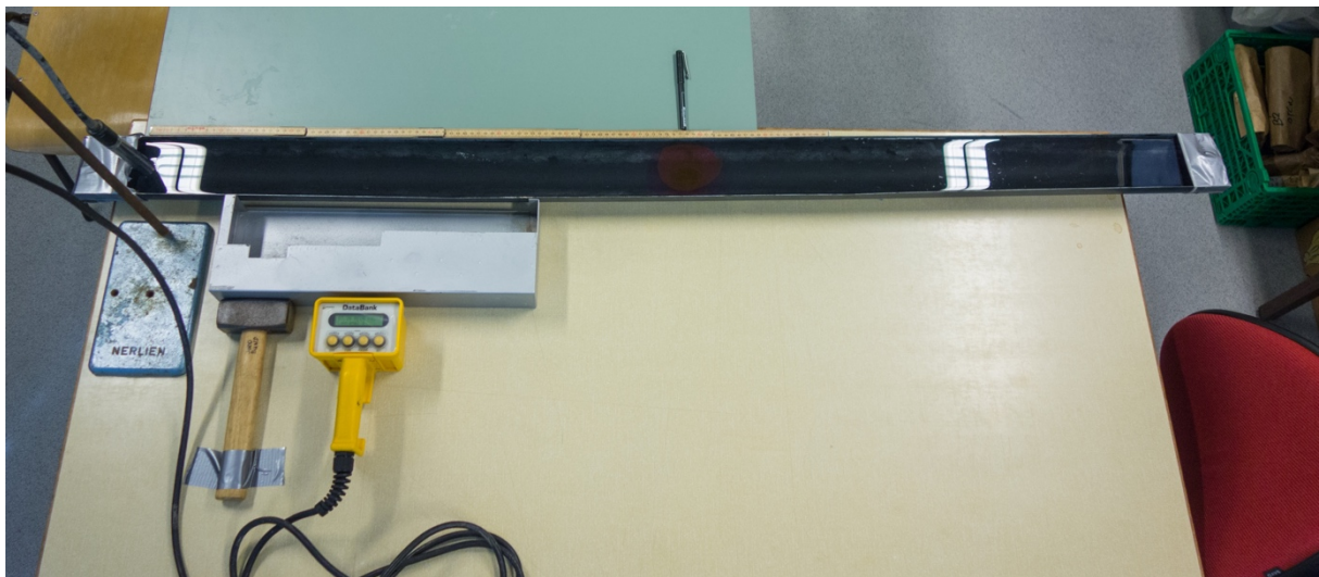
Figure 3.8 The setup for diffusion experiment #1, with stagnant water in the gutter and the Cyclops 7 placed at the far end. The image is taken five minutes after injecting 10 \mu l Rhodamine WT in the center of the gutter. Photo: Jan Hedges
