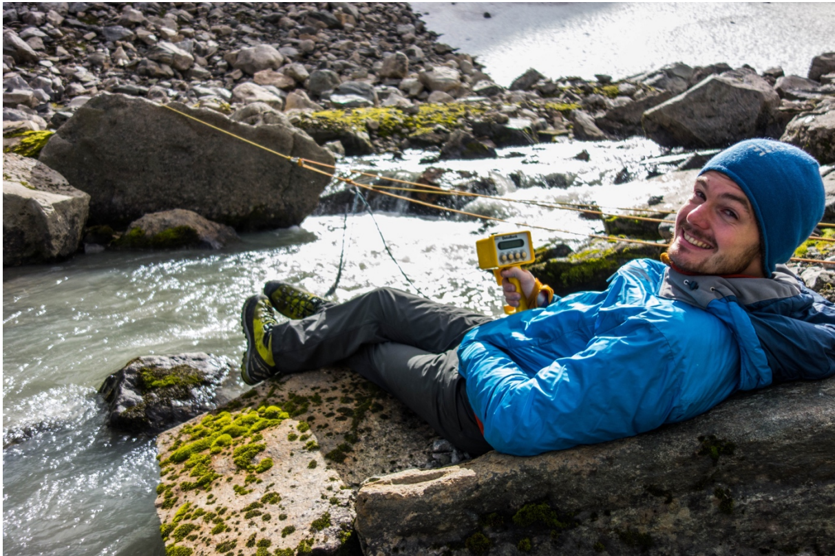
Figure 3.6 The fluorometer in use. Anders is holding the DataBank, while the Cyclops 7 is submerged in the proglacial stream. Photo: Jan Hedges
