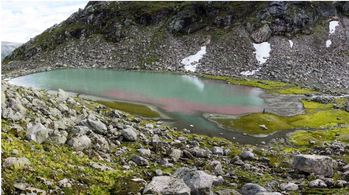
Figure 5.9 Overview image showing dye entering and spreading along the sides of the valley lake during field measurement Lake #4. Photo: Jan Hedges
