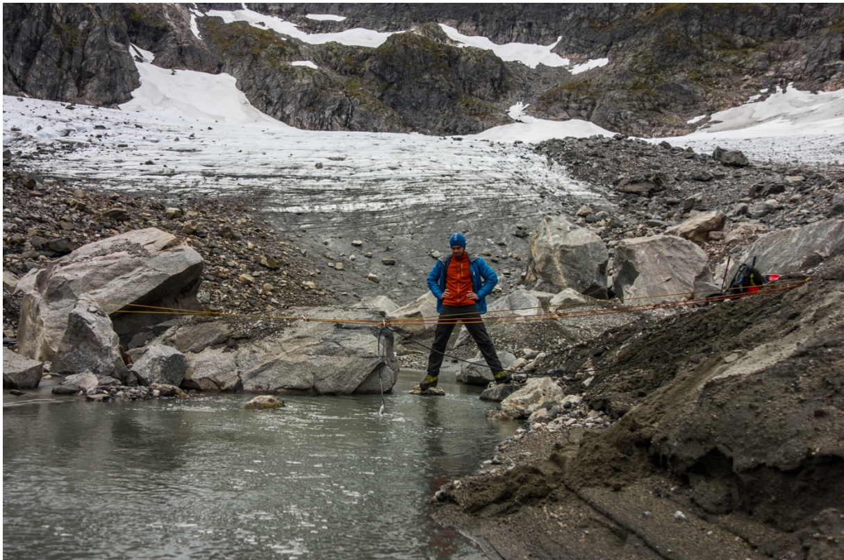
Figure 3.17 The fluorometer setup at MP2, directly below the glacier. The supraglacial stream can barely be spotted; it is located to the left of the large debris-pile in the upper right quadrant of the image. The dye was injected at IP3, which is located a short distance above the same large debris pile. Photo: Jan Hedges
