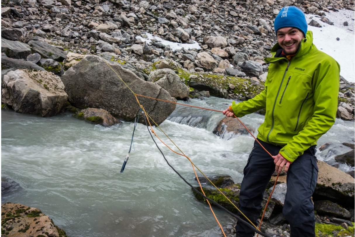
Figure 3.14 This image shows how the Cyclops 7 was positioned in the stream, through use of a rope system attached on either side of the stream. Photo: Jan Hedges
