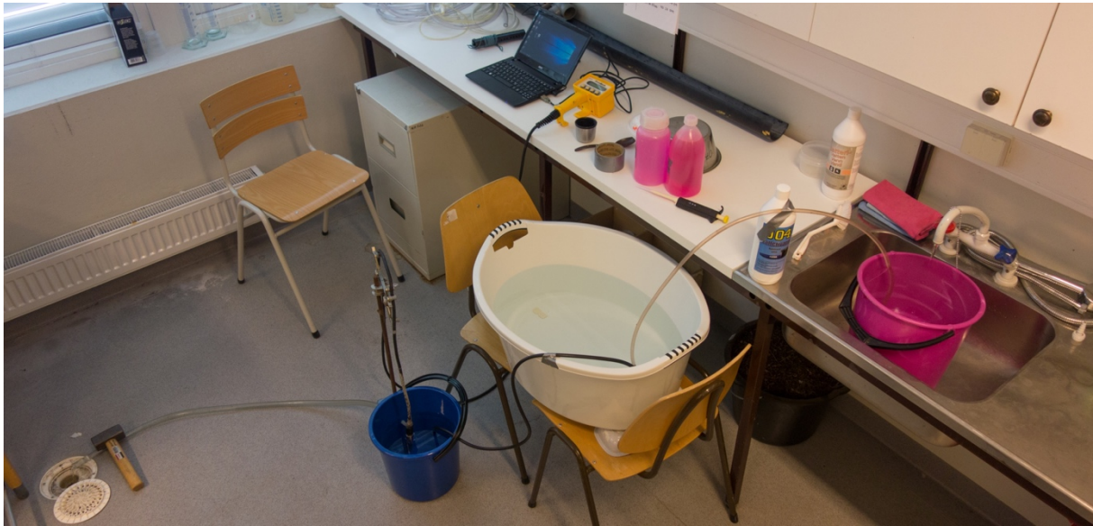
Figure 3.10 This image shows the actual setup of the Siphon experiment. The pink bucket (1), the white tub (3) and blue bucket (5), with siphons connecting them.
