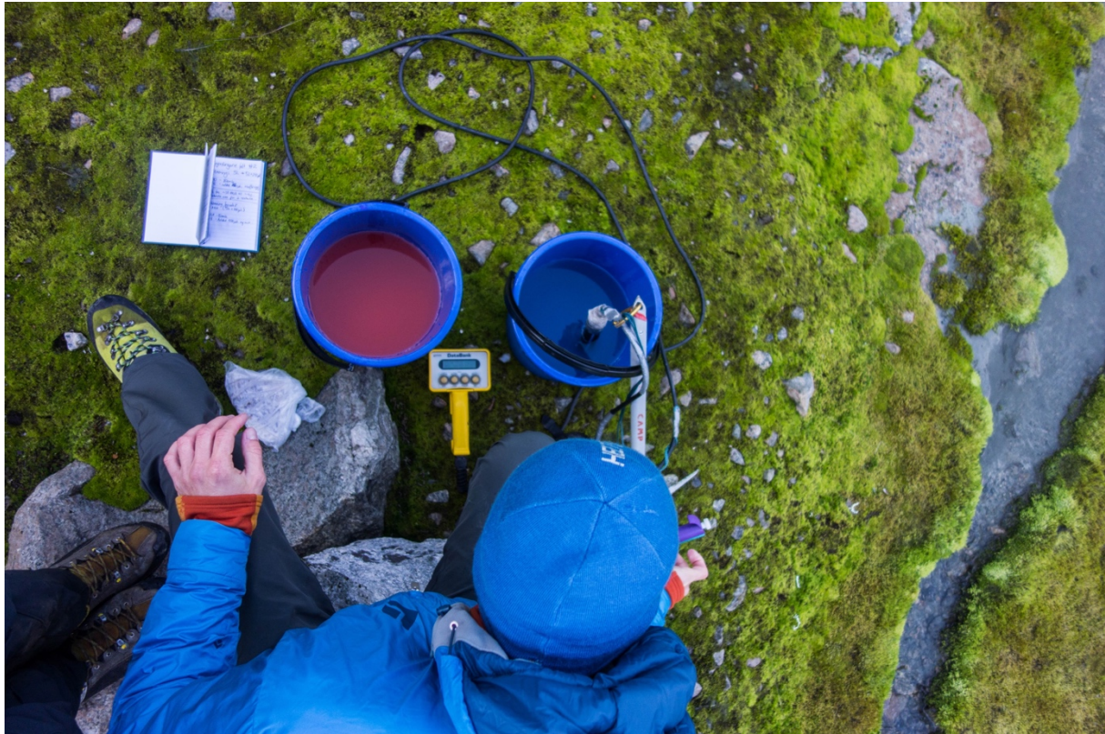
Figure 3.7 The image shows the set up for the calibration procedure (here performed in Skjerdingane). Bucket (1) is to the left and bucket (2) to the right. The DataBank is in the centre, and the Cyclops 7 is suspended in bucket (2). Photo: Jan Hedges
