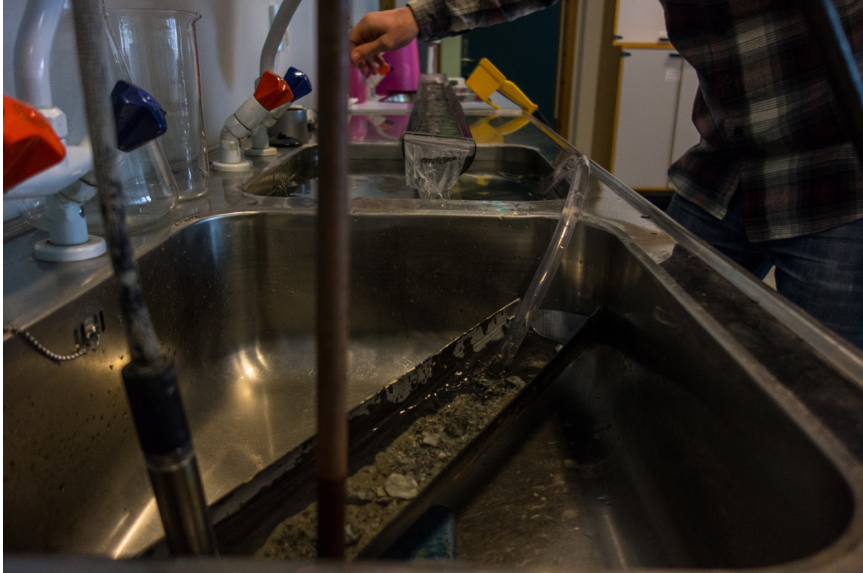
Figure 3.12 An image showing the stream and basin experiment, as seen from above measuring point C2. The initial gutter (1) is seen at the back of the image, the basin (2) and siphon (3) in the middle, and the final length of gutter (4) in the front. Photo: Jan Hedges
