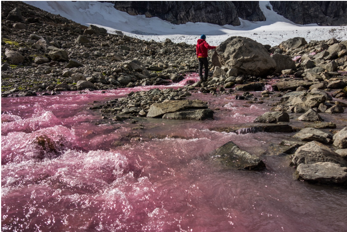
Figure 3.16 The dye concentration close to the injection points is clearly visible. The image also illustrates the typical width and depth of the proglacial stream. Photo: Jan Hedges
