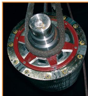
Special rotor design allows extended motor control in Constant Power speed range
