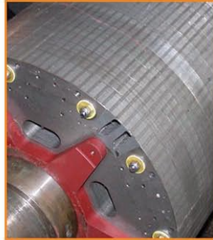
PM segments embedded inside the rotor structure
