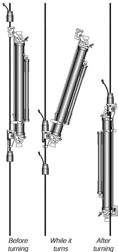
Figure 14: Trapping water with the Nansen Bottle (Nichols & Williams, 2008).
