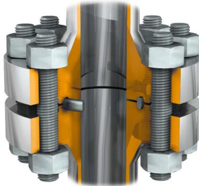
Figure 8 - Example of a bolted flange [16]
