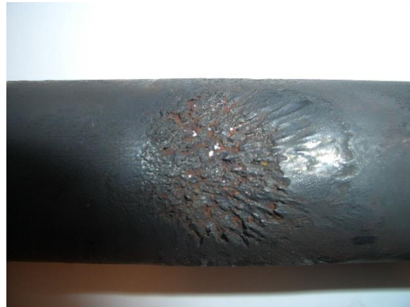
Figure 12 - Damages due to cavitation and erosion 8
