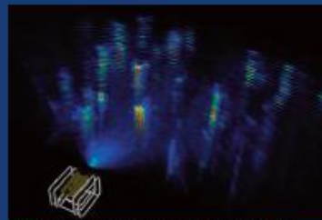
3D Volume Visualisation of underwater pilings
