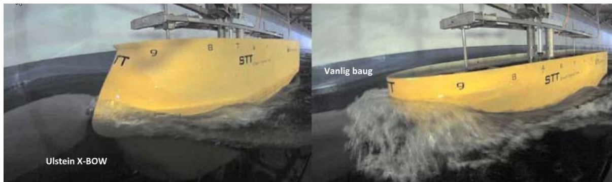
Figur 15 Ulstein (u.å.). Ulstein X-BOW
