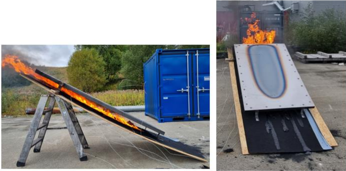
Figure 37: An illustration of the experiment with test setup M4; UL B-crib and PV module.
