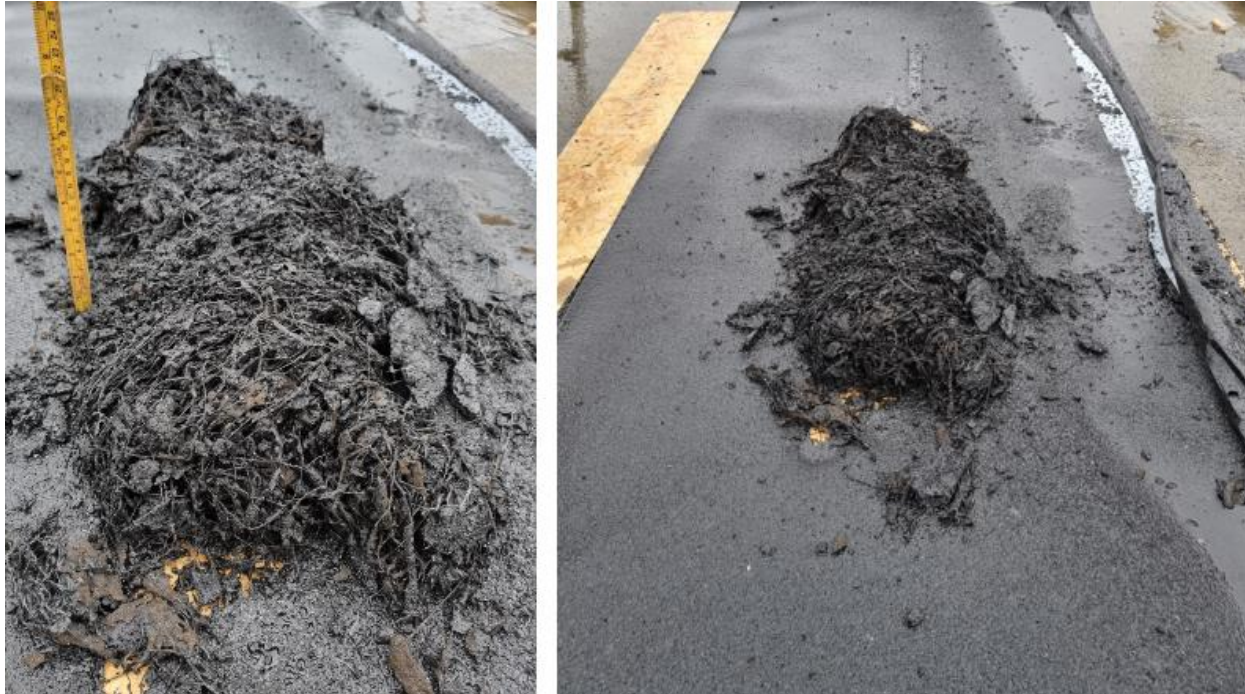
Figure 60: Amount of scraped-off waste from burned roofing membrane after one of the full-scale experiments. Additionally, there was melted roofing membrane on the ground that is not included in this waste
