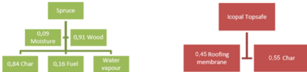
Figure 31: Representation of spruce and Icopal Topsafe's single reaction scheme
