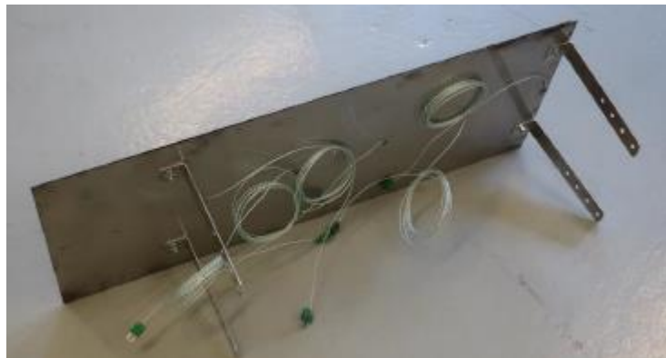
Figure 12: Picture of the mock-up PV module used in the small-scale experimental setup. The mounting brackets and thermocouples are attached on top of the plate. The image is sourced from Stølen et al.[3], p. 11
