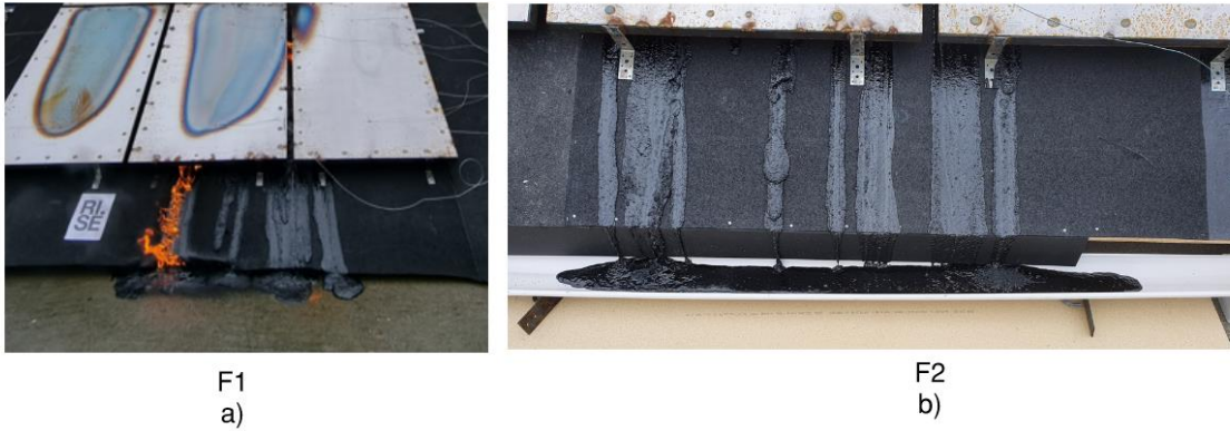
Figure 41: Illustration showing the melted roofing membrane at the eaves in both experiments. In experiment F1 a) the roofing membrane was collected on the ground, while in experiment F2 b) the roofing membrane was collected in a gutter. Only in experiment F1 did the fire spread downwards in the roof construction.
