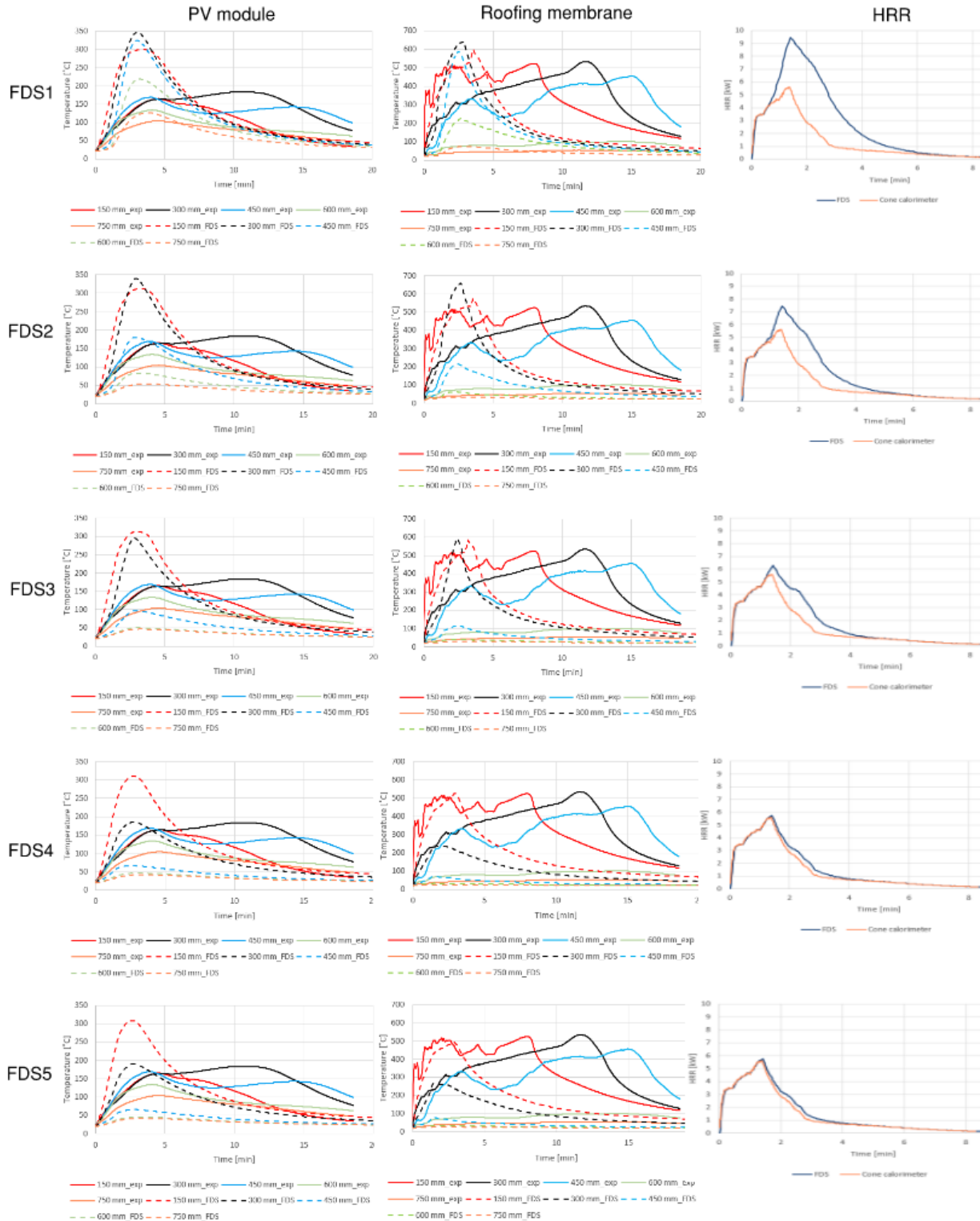
Figure 58: Temperature measurements made in the experiment are shown with solid lines, while dashed lines represent measurements made in FDS. The exception is measurements of HRR where the orange line is data from the cone calorimeter test and the black line is data from FDS. The x-axis shows time (min) and the y-axis shows temperature (°C)/HRR (kW). Both x-axis and y-axis are common for all figures in the same column.
