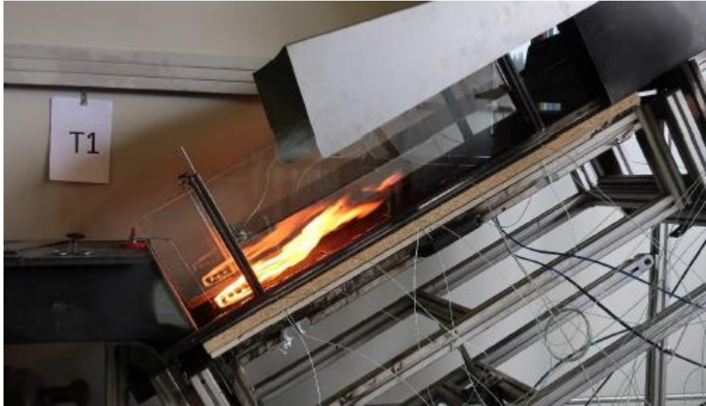
Figure 11: Illustration of the experimental setup used for the small-scale experiments with the PV panel positioned 12cm above the roof surface and with a wind speed of 2m/s. The image is sourced from Stølen et al.[3], p. 10.
