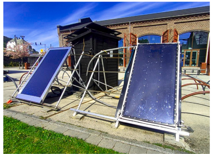
Fig. 1. Flat-plate (left) and DASC (right) mounted on site.
