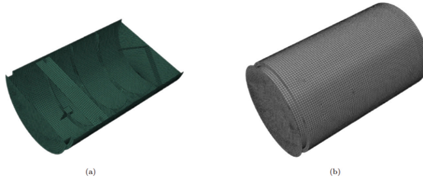
Fig. 8. The FE/BE model of the cylindrical shell, Gao et al. (2022) (a) Finite element model. (b) Boundary element model.
