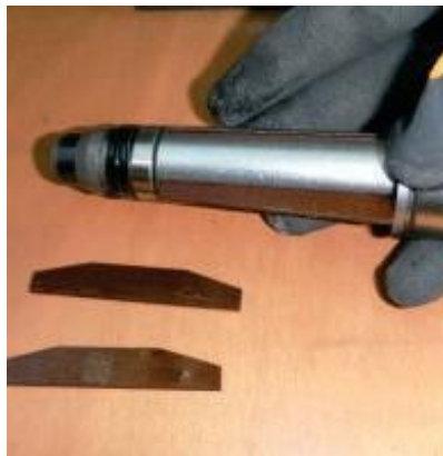
Take the blades out of the pneumatic motor.
