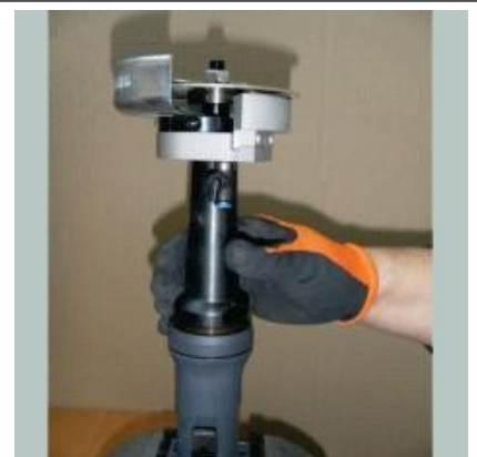
Reassemble the pneumatic cutter and tighten it hand-tight with the spanner.
