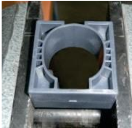
Clamp the holder for the pneumatic cutter in a vice.
