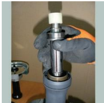
Remove the pneumatic motor and the spacer bushing.
