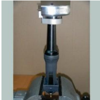
Clamp the tool in the holder.
