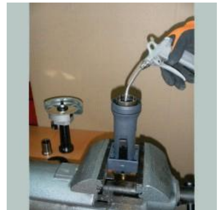
Blow out the housing and motor with compressed air.
