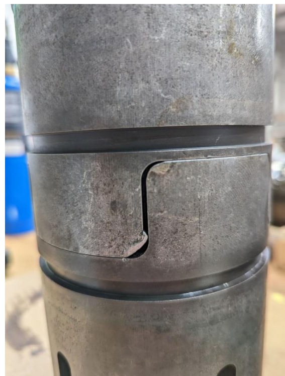
Picture 2 Deformation Side View
