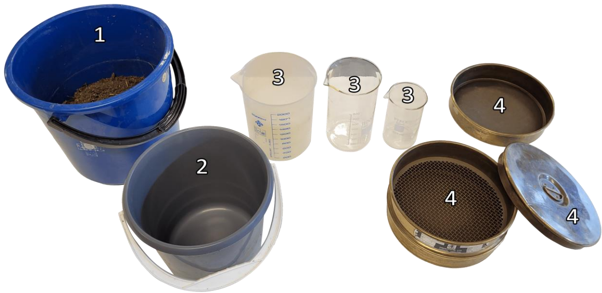
Figure 3. Equipment used for sifting soil samples. 1: Bucket with discarded material. 2: Bucket used for transfer for second sifting. 3: Beakers used for volume registration. 4: 4 mm sieve with bottom pan and top lid.
