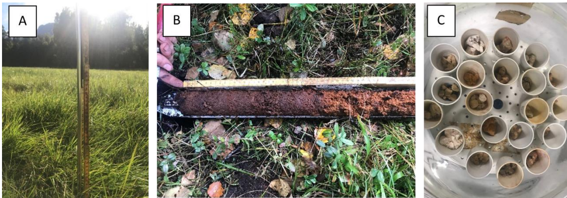
Figure 4. Peat was measured with a peat spear and meter stick (A). Peat cores were brought up by the Russian Corer (B). After loss-on-ignition only ash was remaining in the crucibles (C).
